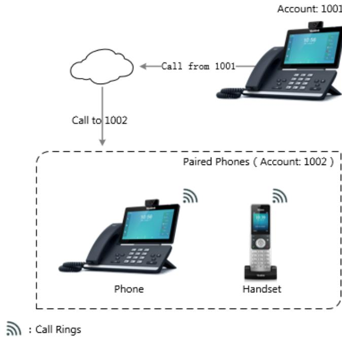
When a call is made from 1001 to 1002, both the phone and the handset ring. Users can answer the call either on the phone or handset.
