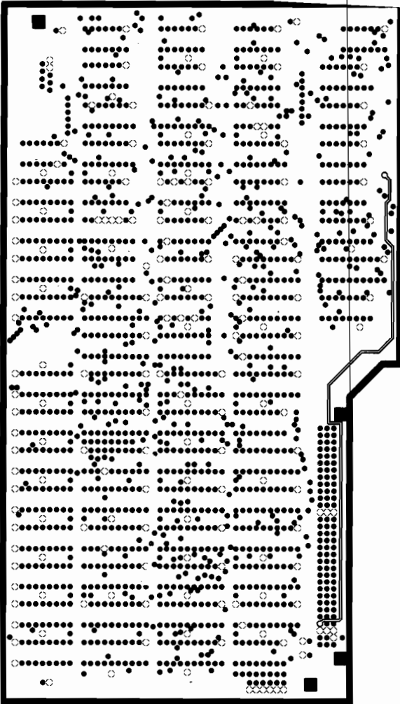
Circuit Trace 1700261, Hi/Lo Res Graphics PCB Ground Plane
