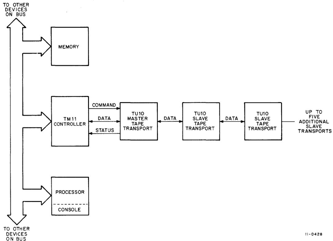
Figure 5-4 TM11 System – Simplified Block Diagram
