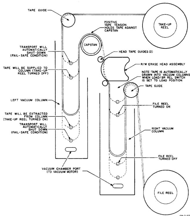
Figure 3-5 Tape Threading
