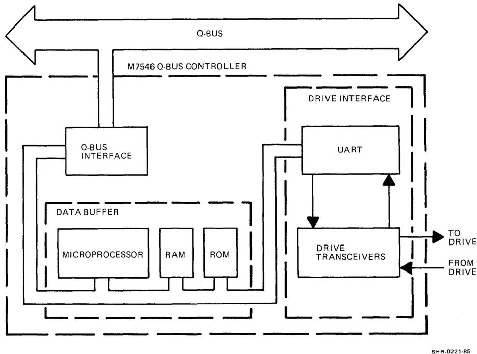
Figure 4-1 TQK50 High Level Block Diagram
