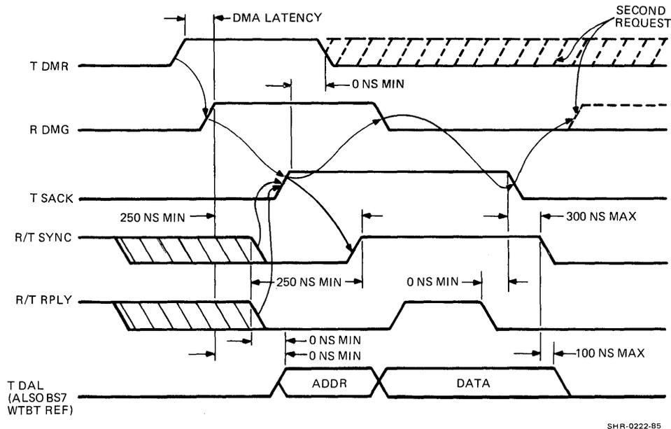
Figure 4-2 Q-bus Timing
