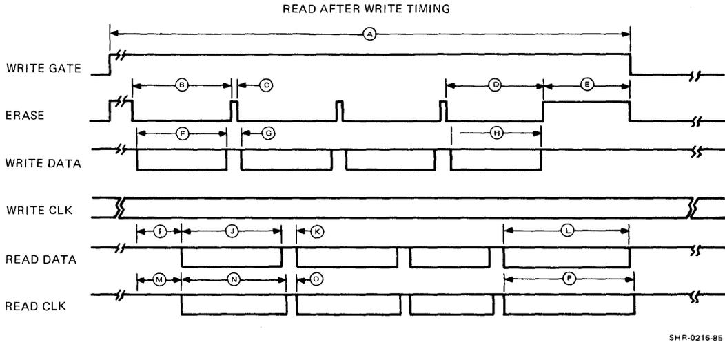
Figure 2-9 Signal Interface Timing (A-P)
