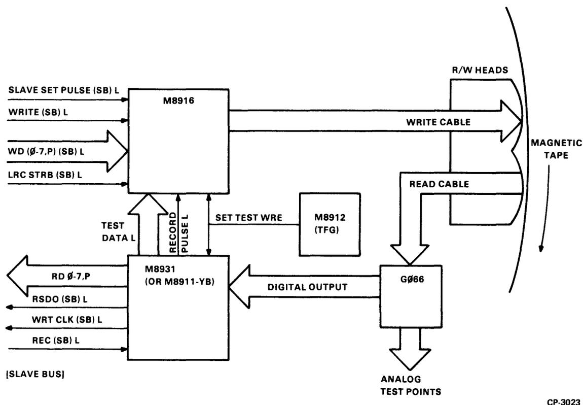
Figure 5-5 Read/Write Functional Block Diagram
