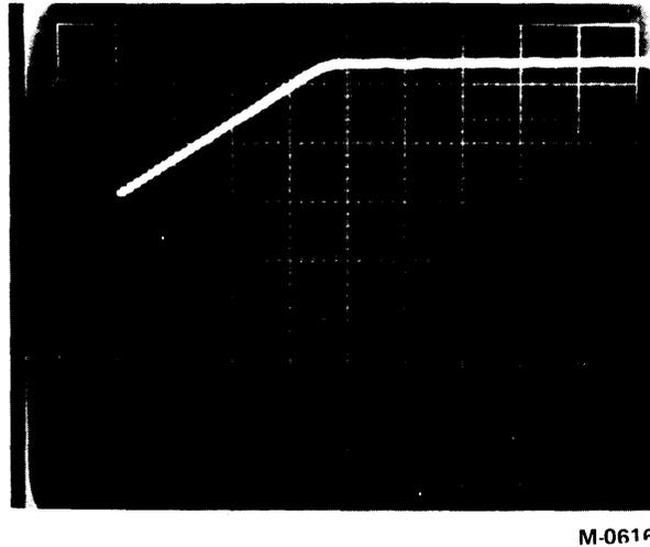
Figure 6-15 Reverse Acceleration Ramp
