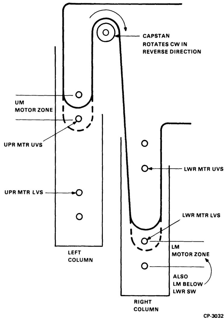
Figure 5-10 Tape Loop Location – Reverse (and Rewind) Motion
