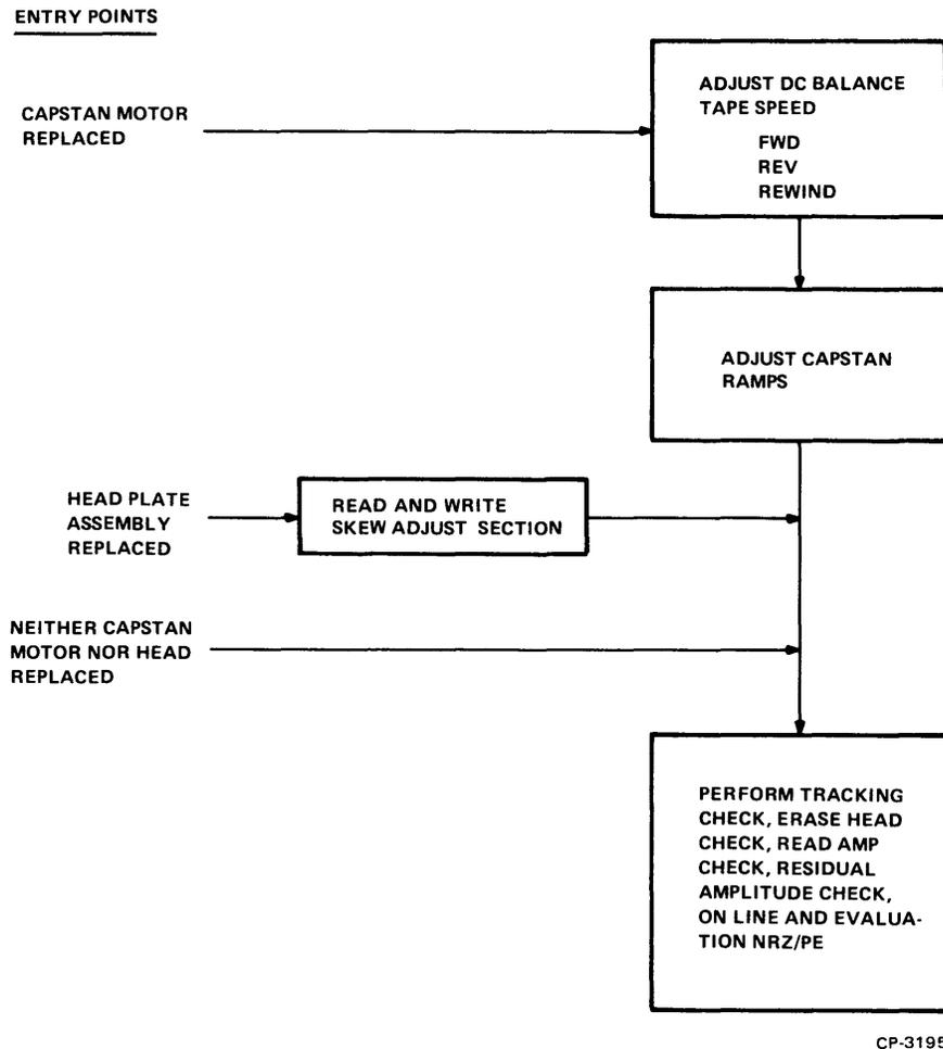
Figure 6-41 Summary, Capstan Alignment Flow Diagram
