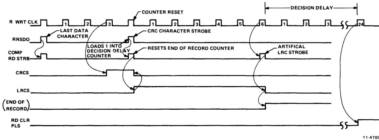
Figure 5-52 End-of-Record Timing, Zero LRC
