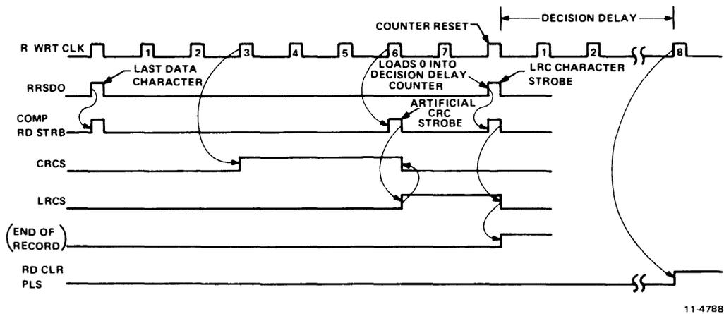
Figure 5-51 End-of-Record Timing, Zero CRC
