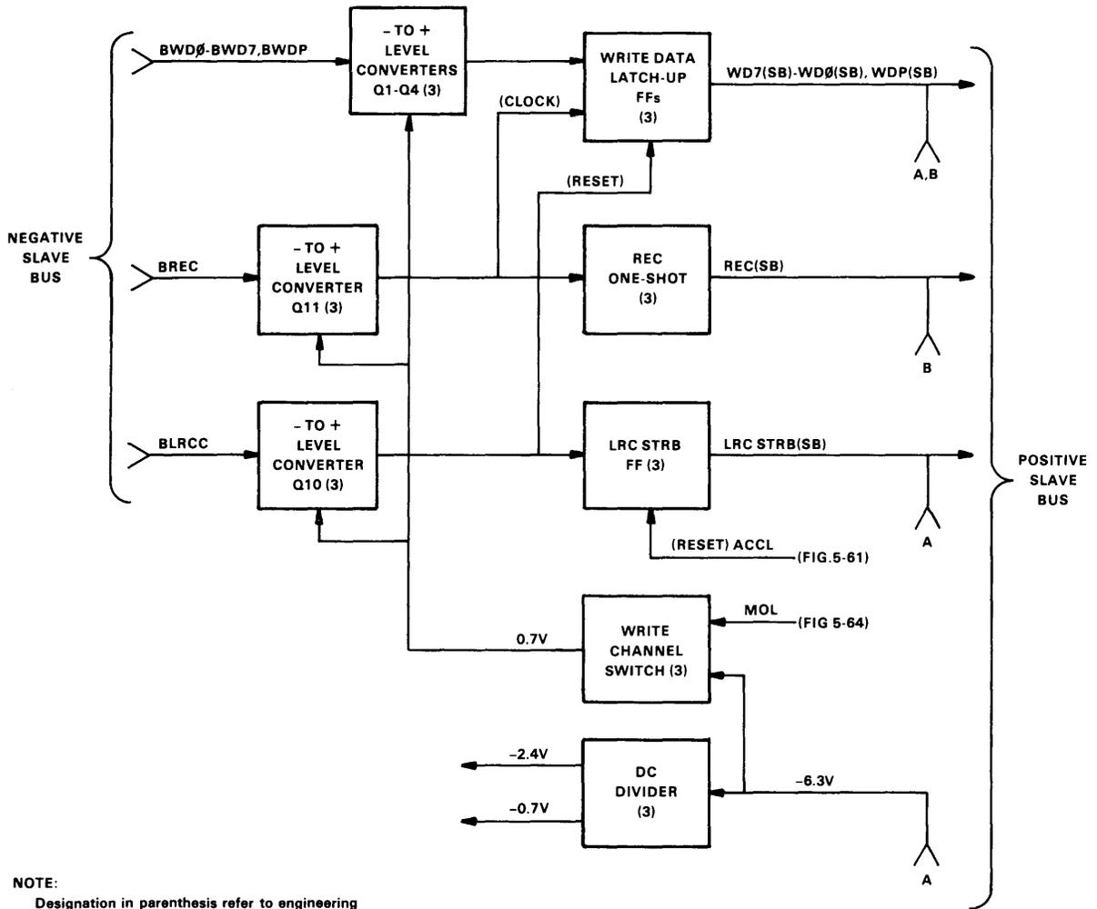
Figure 5-63 Write Data Interface Block Diagram
