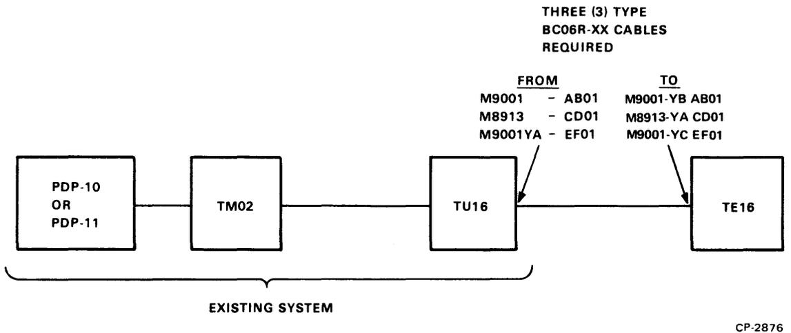
Figure 2-6 Adding Transports to Existing Massbus System
