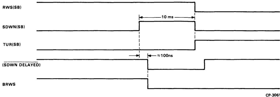
Figure 5-60 RWS(SB) and BRWS Timing Diagram
