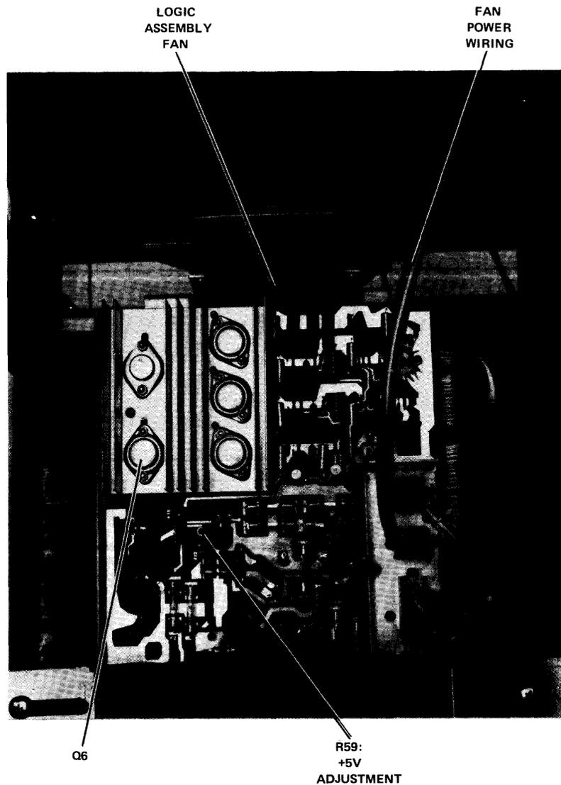
Figure 5-12 TE16 Power Supply Regulator Board (Cover Removed) and Fan
