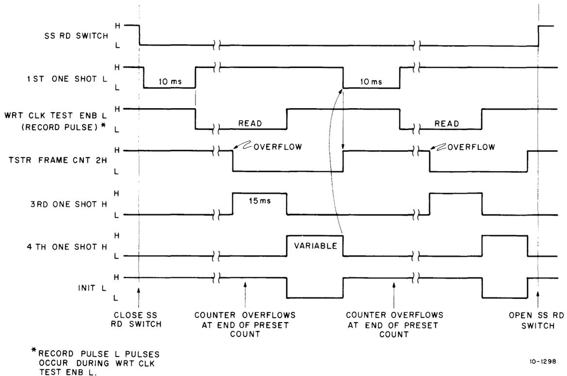
Figure 5-29 SS RD Function Timing
