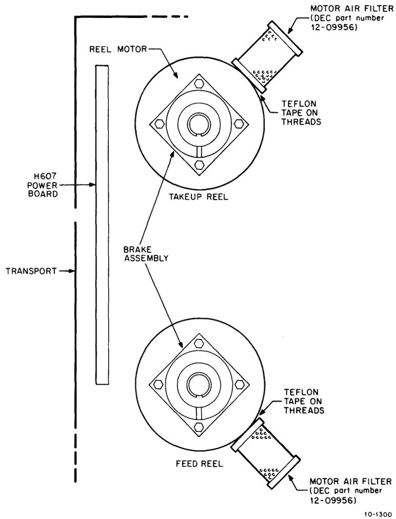
Figure 6-62 Rear View, Reel Motors
