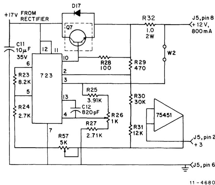
Figure 5-16 +12 V Regulator Circuit (Write Circuits)
