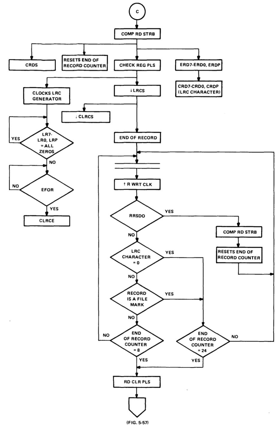
Figure 5-55 End-of-Record Flow Diagram
