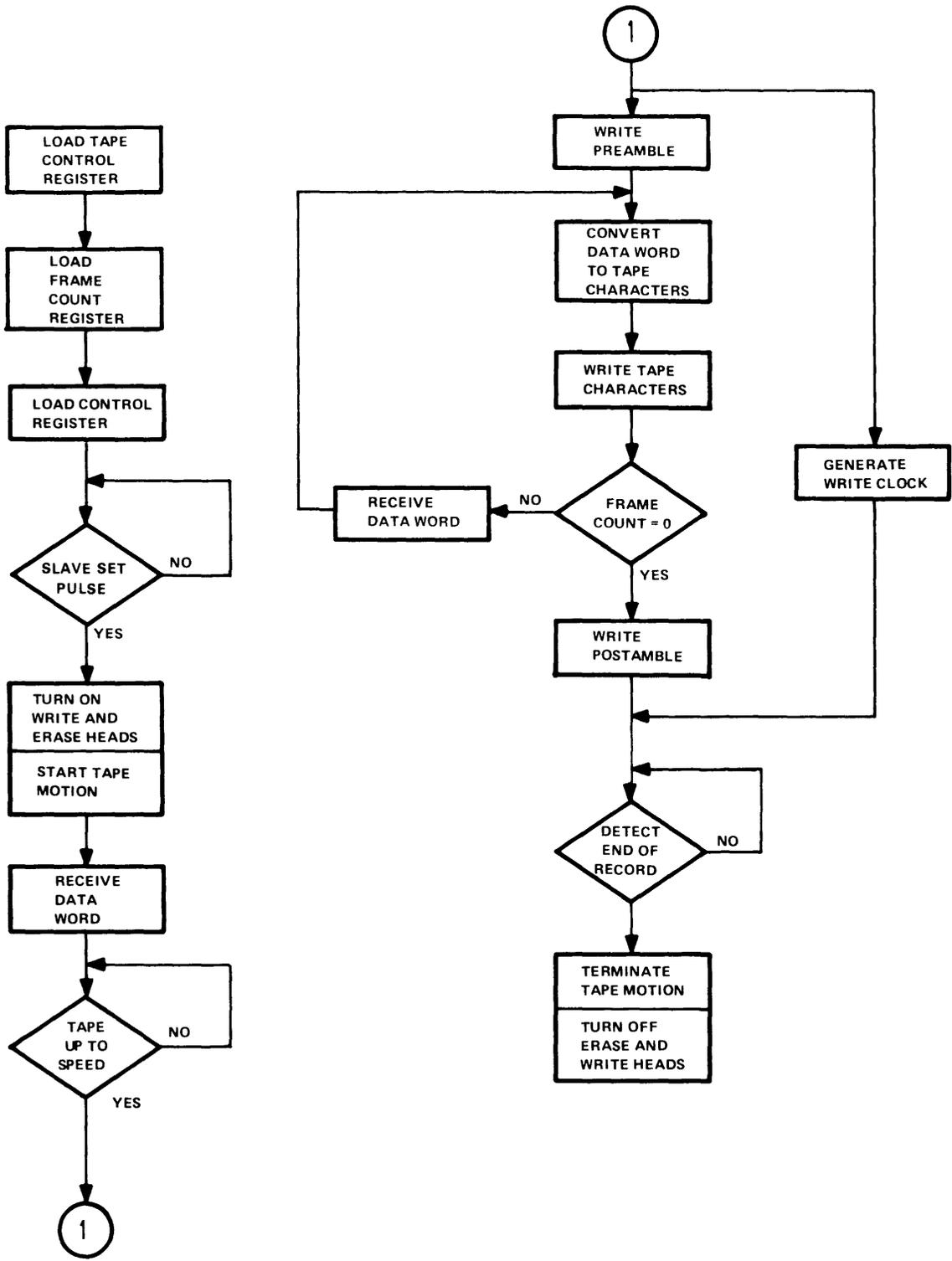
Figure 5-67 PE Data Write Operation Flowchart
