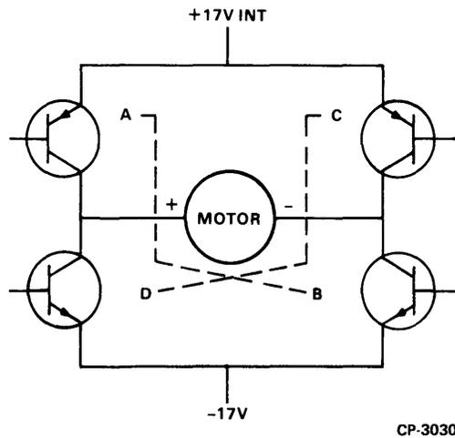
Figure 5-8 Reel Motor Amplifier Equivalent Circuit
