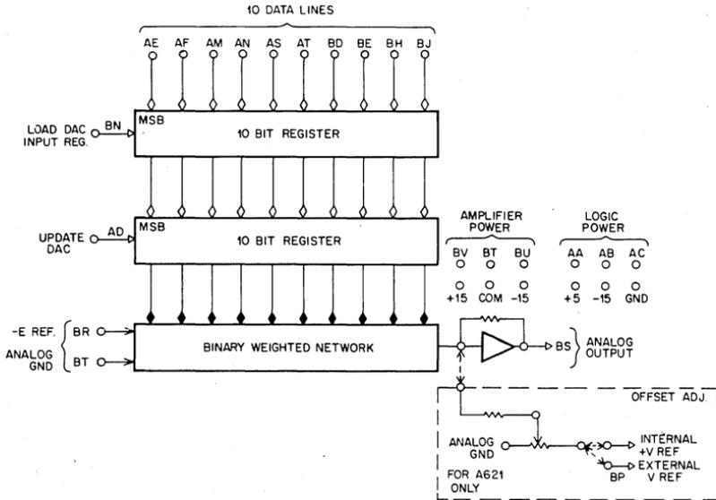
The A620 and the A621 Digital-to-Analog Converters (DAC) are contained on one DEC double Flip-Chip Module. These modules are also double-width in the lower (B section) half. The converters are complete with two 10-bit buffer registers, level converters, a precision divider network, and a current summing amplifier, capable of driving external loads up to 10 ma. The reference voltage is externally supplied for greatest efficiency and optimum scale-factor matching in multi-channel-application.
