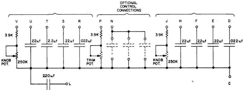
The K432 Timer Control module used with a K301, K303, or K323 allows timer delays to be adjusted from a front panel by rotating a knob-pot. Timing ranges are selected by connecting the desired capacitor as shown in the table below either with wire wrap or 913 grip clip patch cords.
