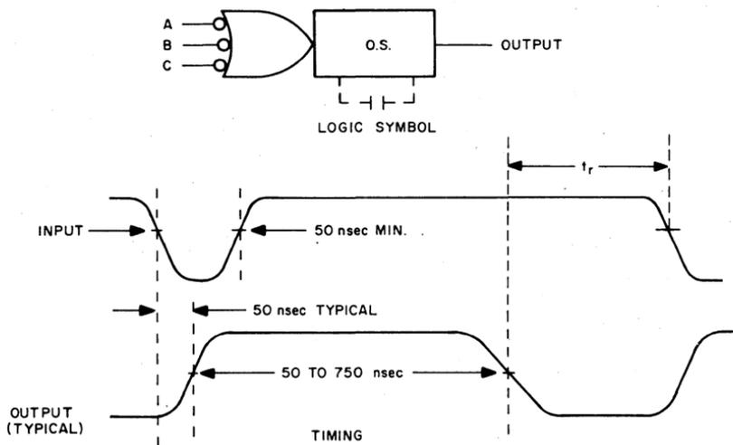
Figure 21. One-Shot Delay Timing and Logic Symbol
