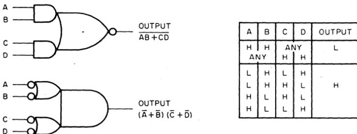
Figure 10 AND/NOR Gate Logic Symbols and Truth Table
