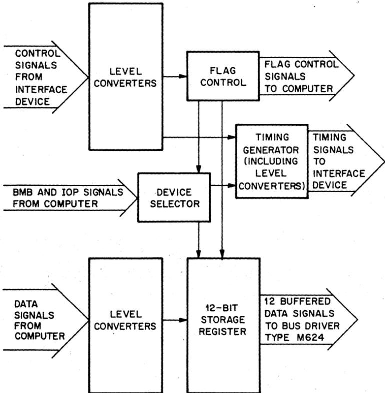
Figure 1. PDP-8/I, PDP-8/L, I/O INPUT BUS INTERFACE MODULE TYPE M732
