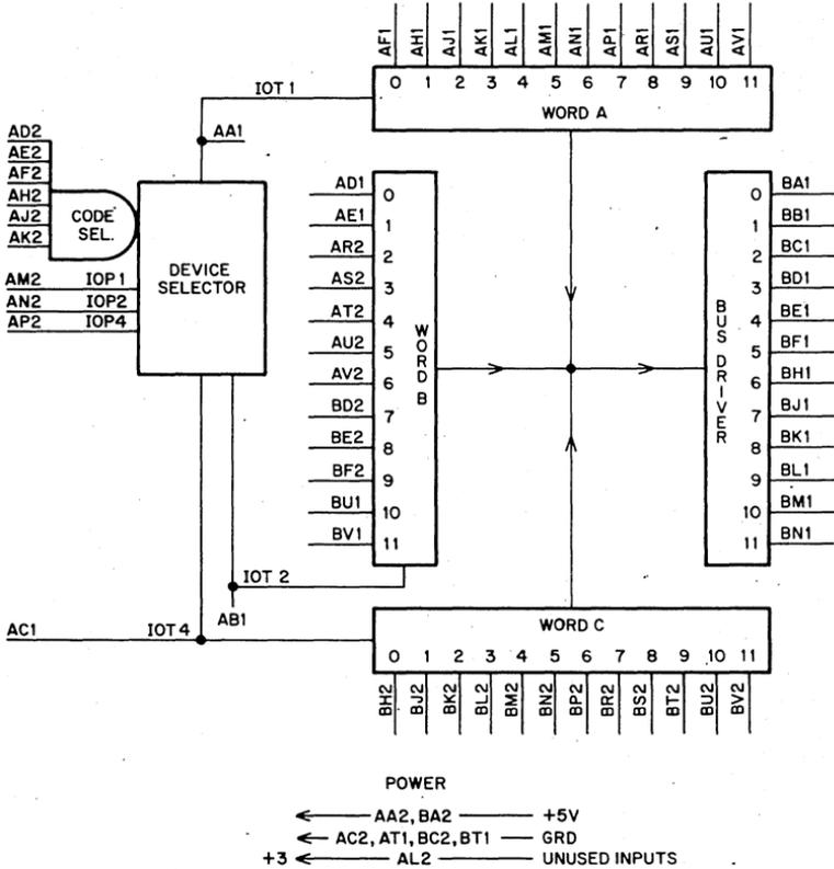
The M734 is a double height, single width module and is a three word multiplexer used for strobing twelve-bit words on the positive voltage input bus; usually the input of the PDP8/I or the PDP8/L. Device selector gating is provided. The data outputs of the M734 Multiplexer consist of open collector npn transistors which allow these outputs to be directly connected to the bus. All inputs present one TTL unit load and function as follows:
