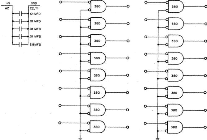
Figure 4 M784 Unibus Receivers\*
