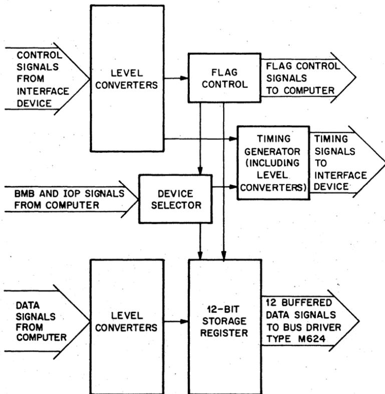
PDP-8/I, PDP-8/L, I/O INPUT BUS INTERFACE TYPE M733
