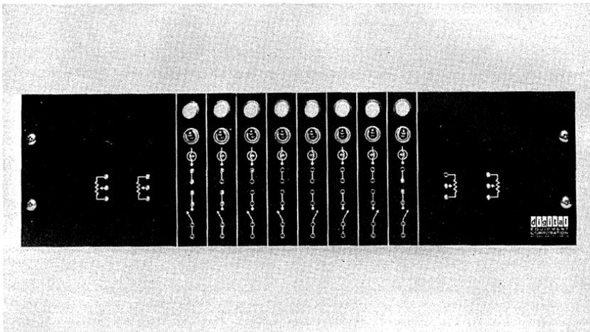
The H902 Panel provides facilities for control and observation of the Logic Laboratory. It contains eight indicator lights and a lamp driver module, eight toggle switches and four potentiometers. Connections to these devices are made with Type 911 Stacking Banana-Jack Patchcords.
