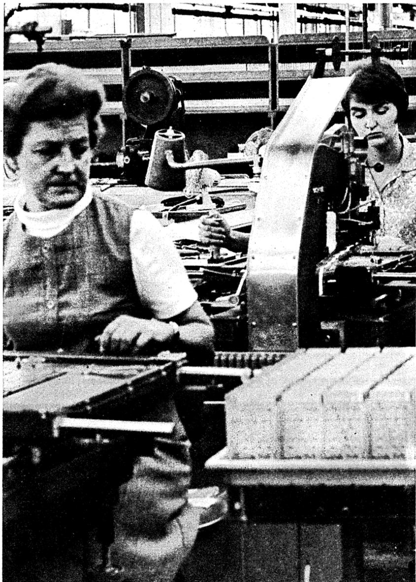
Discrete components for DIGITAL Modules are positioned and crimped in place at rates up to 2,200 per hour on pantograph controlled inserting machines. Board layouts put like parts in rows, minimizing the effort required to follow the template. Several templates for each module type are generated by numerically controlled milling machines.
