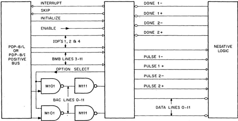
Figure 3: USE OF M731 USING M101 & M111
