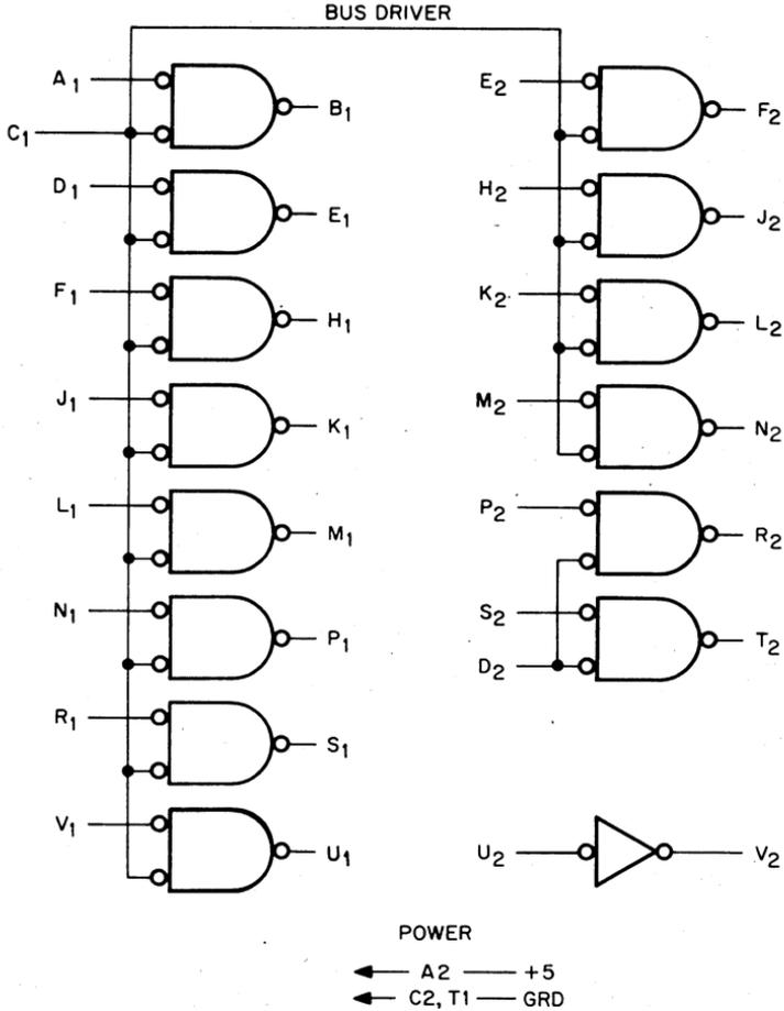
The M624 contains fifteen bus drivers intended for convenient driving of the positive input bus of either the PDP-8I or PDP-8L. Twelve of the drivers have a common gate line and would be used for DATA. There are three additional drivers, two of which share a common gate line and the third without a gate line. These three additional drivers were intended to accommodate the functions of "Program Interrupt", "IO Skip" and "Clear AC".
