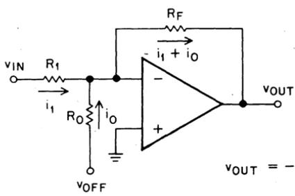
$$v_{OUT} = -v_{IN} \left( \frac{R_F}{R_1} \right) + \underbrace{\left[ -v_{OFF} \left( \frac{R_F}{R_0} \right) \right]}_{\text{OFFSET}}$$
