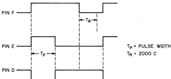
Hysteresis at the inputs makes it possible to use the outputs of the K578, K580 and K581 modules as inputs. The AND expansion node may be used with a K003 to generate pulses from a counter. Even though each pulser may have a different timing capacitor, it is recommended that all circuits be given the same width on all modules so that modules may be interchanged without creating logic timing problems.
