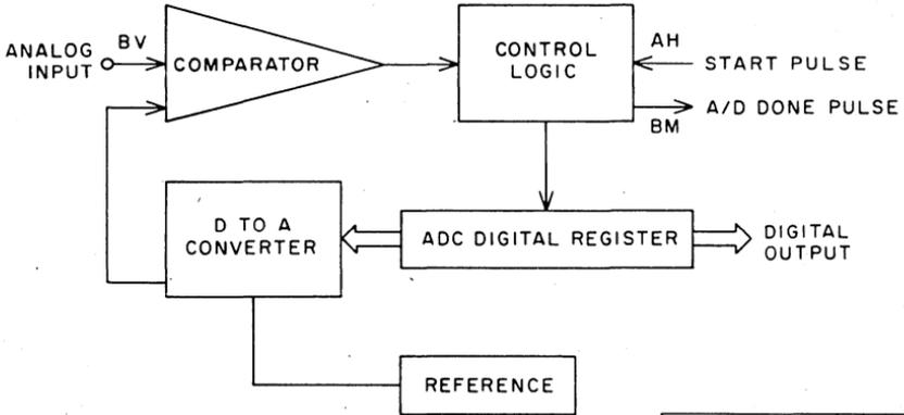
A811 10-BIT ANALOG-TO-DIGITAL CONVERTER
