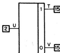
The K501 can be used with the K580, K581, or K578 to provide simultaneous true and complement signals with full K series drive. Built in hysteresis and slowed outputs insure reliable operation in noisy signal environments.
