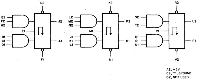
The M202 contains three J-K flip-flops augmented by multiple-input and gates. For general use as gated control flip flops or buffers.
