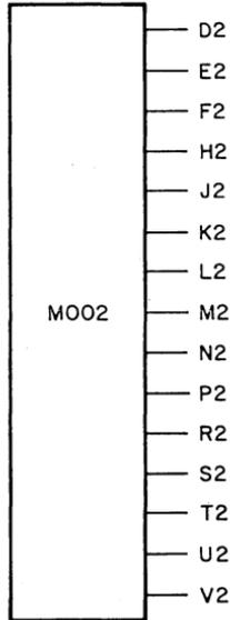
To hold unused M-Series TTL gate inputs high, the M002 provides 15 outputs at +3 volts (Logic 1), on pins D2 through V2. Up to 10 unused M-Series gate inputs may be connected to any one output. If a M002 circuit is driven by a gate, it appears as two TTL unit loads or 3.2 ma. at ground.
