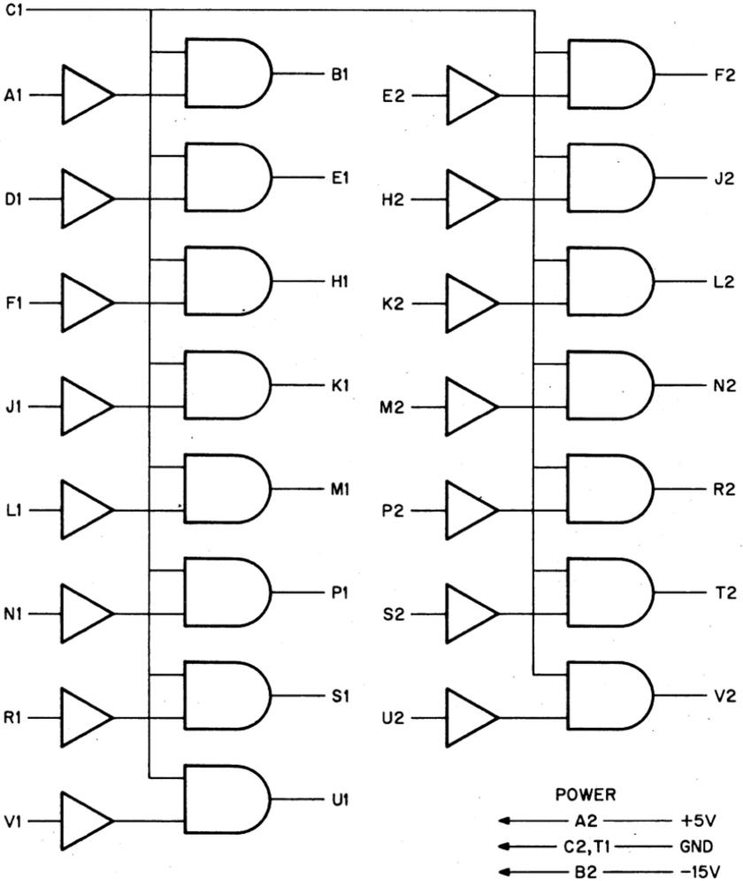
The M100 Bus Data Interface contains fifteen circuits for convenient reception of data from the PDP-8, PDP-8/I negative voltage bus. It is pin compatible with the M101 Positive Bus Data Interface.
