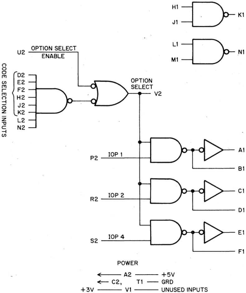
The M103 is used to decode the six device bits transmitted in complement pairs on the positive bus of the PDP8/I and PDP8/L. Selection codes are obtained by selective wiring of the bus signals to the code select inputs D2, E2, F2, H2, J2, and K2. This module also includes pulse buffering gates for the IOP signals found on the positive bus of the above computers. Two two-input NAND gates are also provided for any additional buffering that is required.
