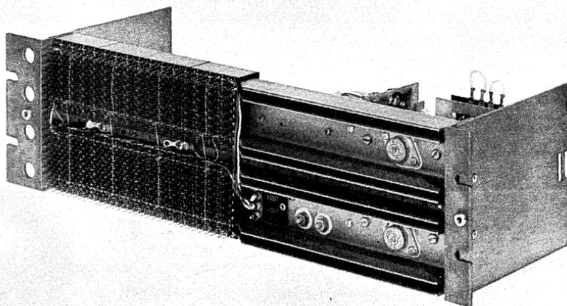
The dual function mounting panel offers a way to build complete digital systems of up to 32 FLIP CHIP modules into only  $5\frac{1}{4}$  inches of rack space. More power is available than is ever likely to be consumed in a 32 module system. Power in excess of that required for modules can be obtained at the H022 terminal block which is conveniently located for connection to the input H022 terminal block on any adjacent H911 or 1943 mounting panel.
