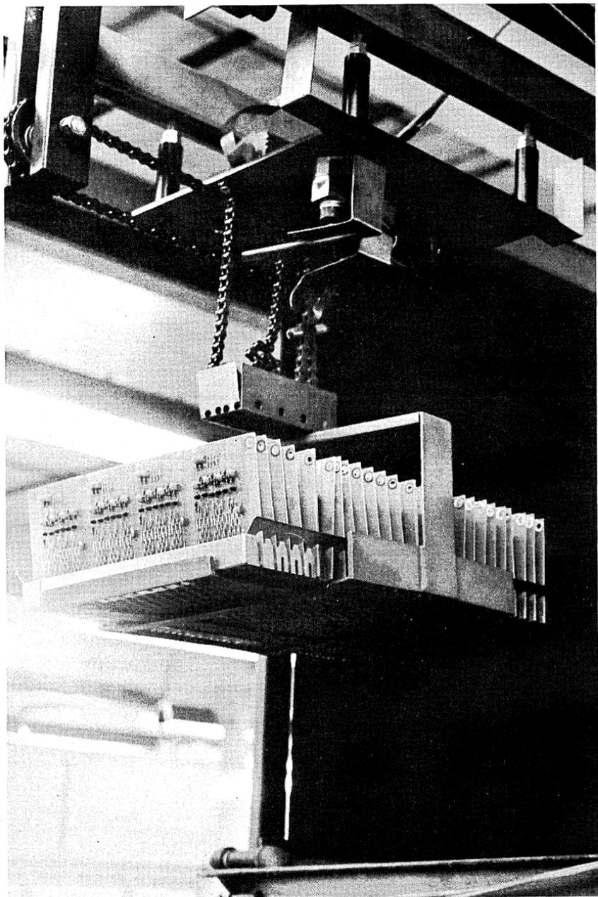
After all the components have been attached to the board, the module is degreased to remove contaminants in preparation for flow soldering.
