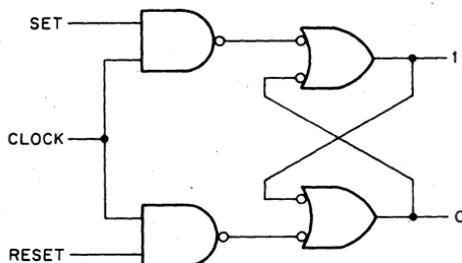
Figure 13 Clocked NAND Gate Flip-Flop
