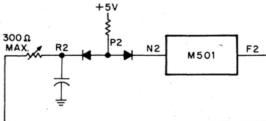
**Inputs:** Input signal swing on PIN R2 is limited to  $\pm 20$  volts.
