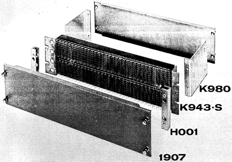
These low cost, 19" panels have sixty four, 18 pin connector sockets with either wire-wrap (R) or solder fork (S) contact pins. Shipped with connector blocks installed and pins A and C bussed.
