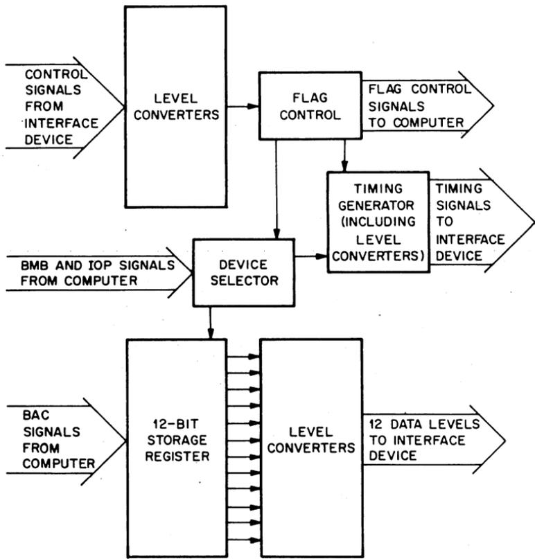
Figure 1. PDP-8/I, PDP-8/L, I/O OUTPUT BUS INTERFACE MODULE TYPE M731
