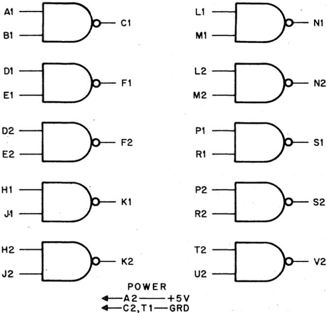
This module provides general purpose high speed gating for the M-Series. Maximum output propagation delay to a logic 1 or 0 is 10 nsec. The high speed characteristic of these gates frequently will solve tight timing problems in complex systems. Unused inputs on any gate must be returned to a source of logic 1 for maximum speed and noise immunity.
