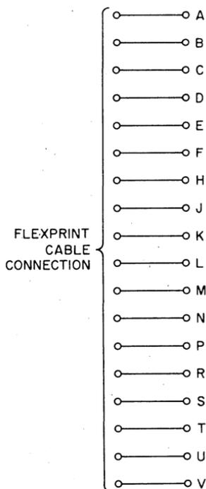
The K080 cable connector consists of a single height, single thickness board on which can be mounted a 19 conductor flexprint cable. Each module comes with a cable clamp for customer convenience.
