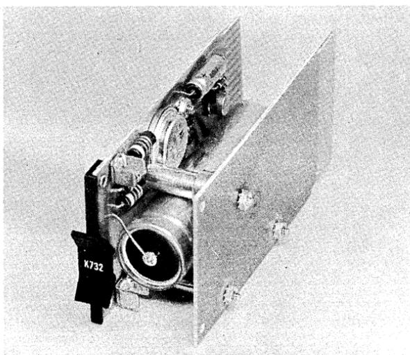
One K731 plus up to 3 K732 can provide from 1 to 7 amperes at +5v.
