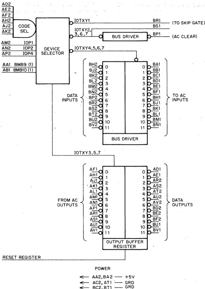
The M735 provides one 12-bit input bus driver and one 12-bit output buffer register for input and output data transfers on the positive I/O bus of either a PDP8/I or a PDP8/L. Device selector gating plus additional signal lines provide the flexibility necessary for a complete interface with the exception of flag sense signals. Use of the M735 is not restricted to a computer, as it can be used in many systems to provide reception and transmission of data over cables.
