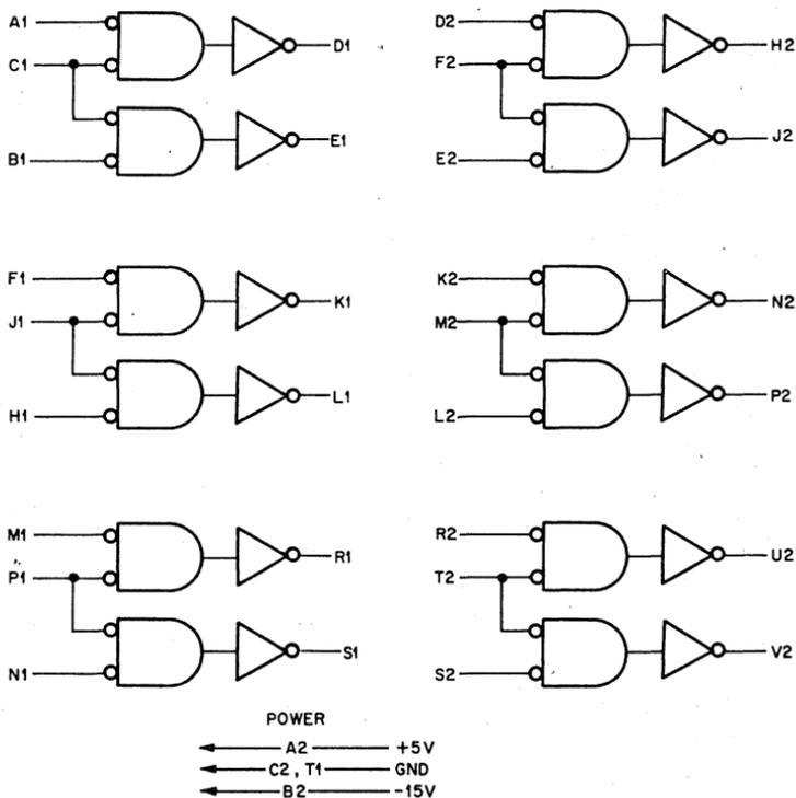
The M633 contains twelve bus drivers intended for convenient driving of the negative bus of the PDP-8, PDP-8/I. Each driver consists of an open collector PNP transistor. It is pin compatible with the M623 positive voltage bus driver.
