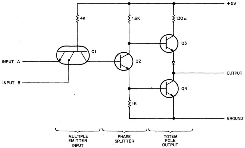
Figure 1 TTL NAND Gate Schematic Diagram
