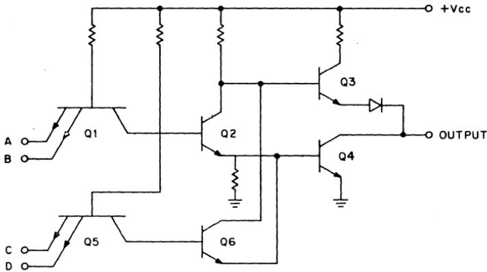
Figure 9 TTL AND/NOR Gate Simplified Schematic
