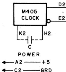
The M405 clock employs a series resonant crystal oscillator to obtain a frequency stability of .01% of specified value between 0°C and +55°C. The clock frequency may be specified anywhere in the range of 5 KHz to 10 MHz by the customer.
