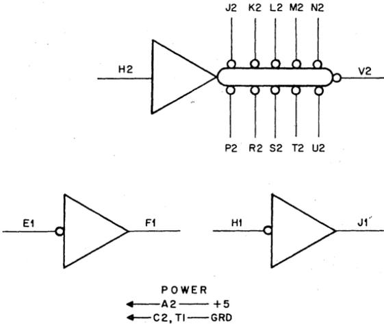
The M310 consists of a tapped delay line with associated circuitry and two pulse amplifiers. The total delay is 500 nanoseconds with taps available at 50 nanosecond intervals.
