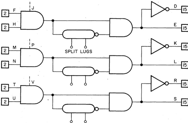
The K333 Pulser circuits are designed to produce pulses from low to high level transitions. The length of a pulse is determined by the capacitance connected to split lugs conveniently mounted on the module.
