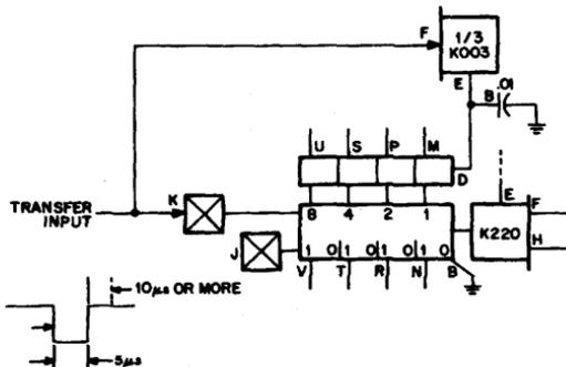
This circuit gives approximately 10 microseconds of rise delay. The delay may be reduced to about 5 microseconds if desired, by connection another one milliamper pull-up (pin D to pin E on the K003).
