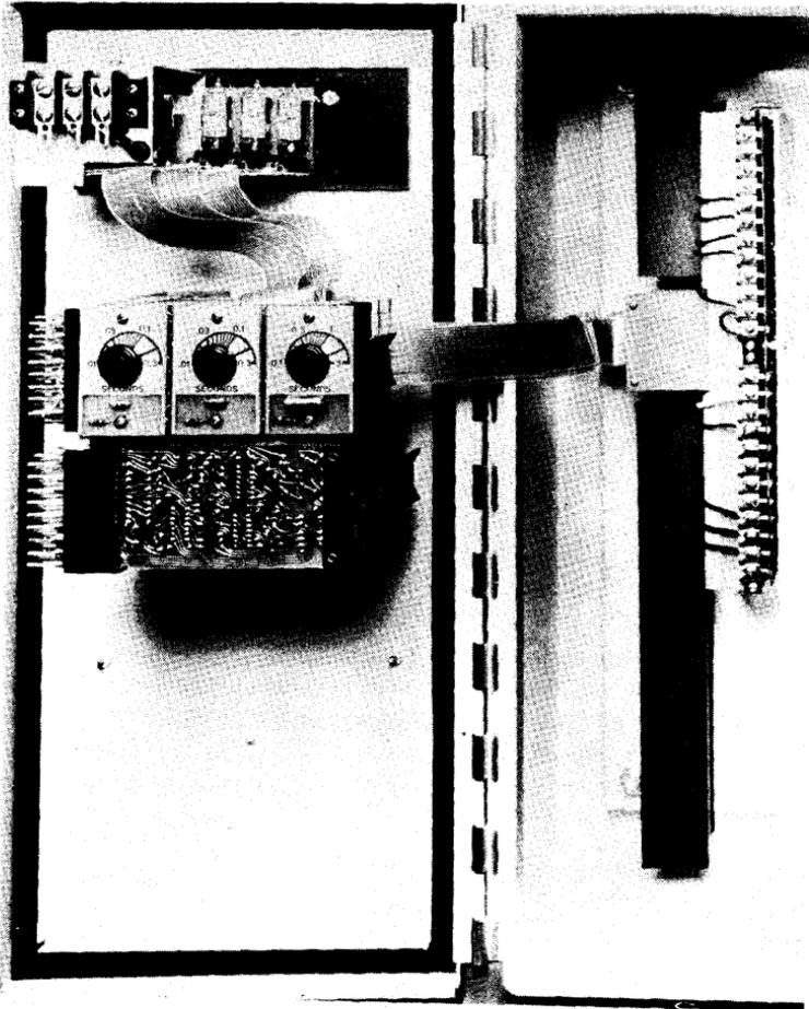
SMALL K-SERIES CONTROL INSTALLED IN NEMA 12 ENCLOSURE.
