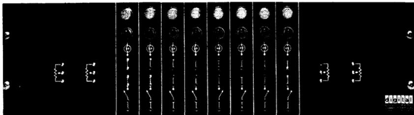
The K902 Panel provides facilities for control and observation of the Logic Laboratory. It contains eight indicator lights and a lamp driver module, eight toggle switches and four potentiometers. Connections to these devices are made with Type 911 Stacking Banana-Jack Patchcords.
