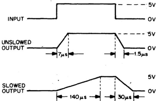
With 5KHz slowdown connected, a noise spike must now maintain the necessary voltage and current threshold levels for 30 microseconds instead of the typical 1.5 microseconds at 100KHz.
