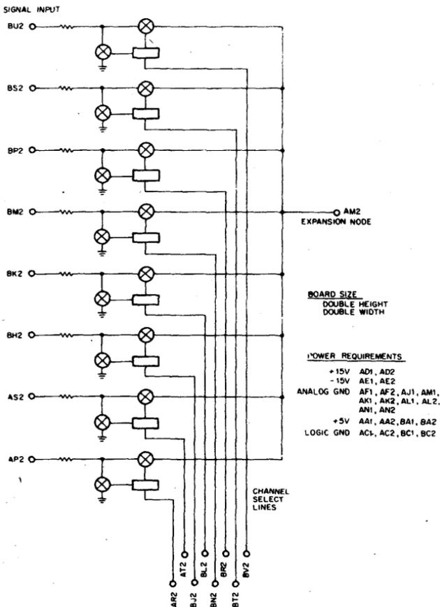
The A164 is an 8 channel constant impedance multiplexer expander utilizing eight FETS to switch the input signal through eight precision resistors either to ground (OFF) or to a virtual ground null point of an operational amplifier (ON).
