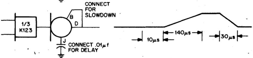
Time shown above are typical values and should not be considered exact. Delay times are increased by 10  $\mu$ s for each .01  $\mu$ f capacitor connected to pin J.
