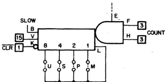
The K211 is a binary counter that can be wired to produce a high to low output transition on pin V after any number of input cycles from 2 to 16. Count-up occurs on the high to low transition of the count gate output.
