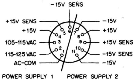
The H704 and H707 contain two 15 volt floating power supplies. To get  $\pm 15$  volt supply, connect pins 7 and 8 and use this point as ground. Pin 4 will now be at positive 15 volts and pin 11 will be negative 15 volts.
