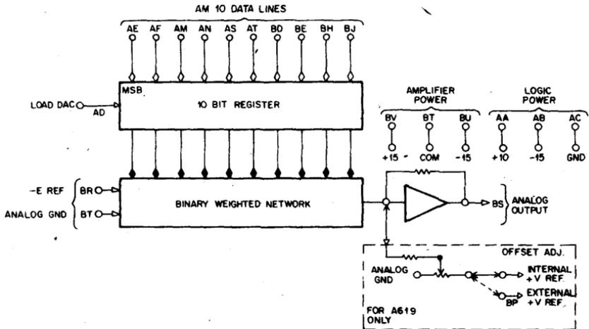
The A618 and the A619 Digital to Analog Converters (DAC) are contained on one DEC double Flip-Chip™ Module. These modules are also double width in the lower (B section) half. The converters are complete with a 10-bit buffer registers, level converters, a precision divider network, and a current summing amplifier capable of driving external loads up to 10 ma. The reference voltage is externally supplied for greatest efficiency and optimum scale factor matching in multi-channel applications.
