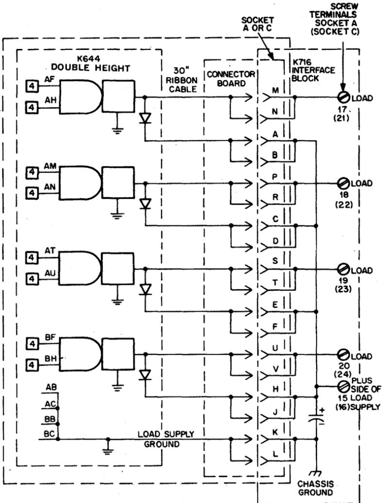
Operating through the K782 or K716 Interface Block, the K644 DC Driver permits stepping motors, dc solenoids, and similar devices rated up to 2.5 amperes at 48 volts to be driven directly from K series logic. Built-in clamping diodes protect switching transistors from transient over-voltage.
