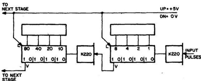
Shown below is a means of acceptance up and down pulse-trains from two separate sources. For this application, input pulse spacing should be at least 20 microseconds and input pulse widths should be at least 10 microseconds.
