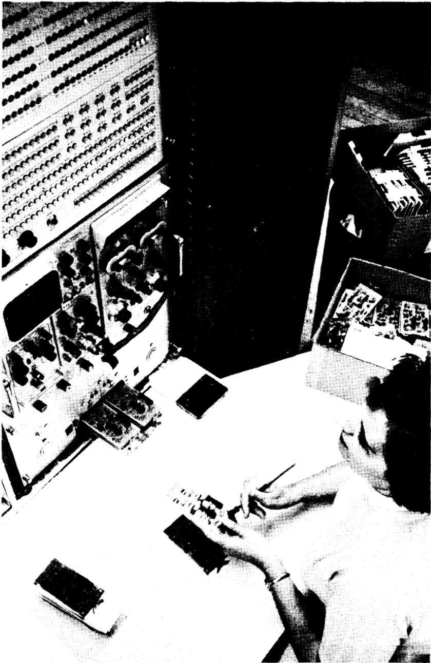
DEC thoroughly tests all finished modules as well as incoming components. Most of the testing is conducted on computerized equipment such as this one which performs 100 ac and dc tests in less than 5 seconds on each module tested.
