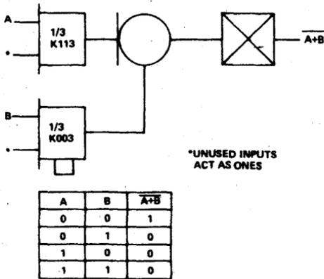
NOR FUNCTION OF BASIC INVERTING GATE WITH EXPANDER
