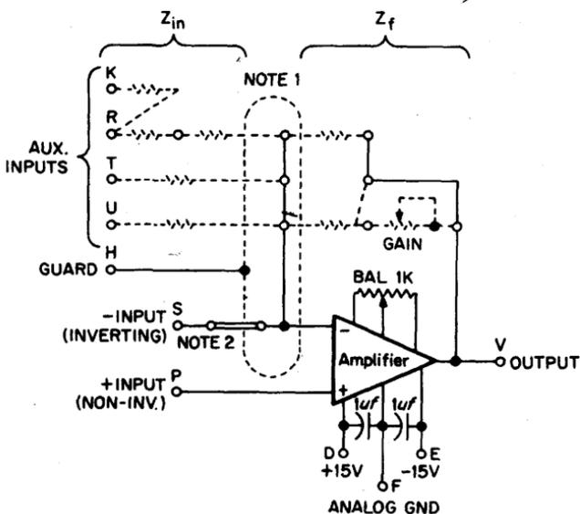
NOTE 1. Mounting holes are provided on the module so that input and feedback components can be added. Components shown with dashed lines are not included with the module.
