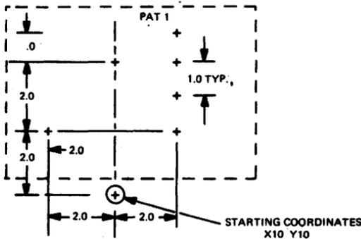
For instance, to define a pattern of random holes, the operator types PAT with an identifying number. All coordinates and geometric commands which follow are included in the pattern definitions until an END command is typed. For example:
