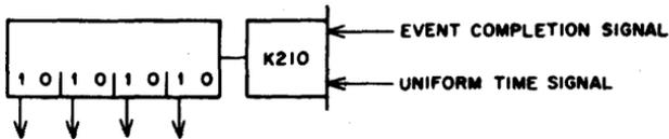
Event completion signal gates the time signal if the latter is a normally low, relatively higher frequency signal. Event completion signal augments the time signal if the latter is a normally high, relatively lower frequency signal.
