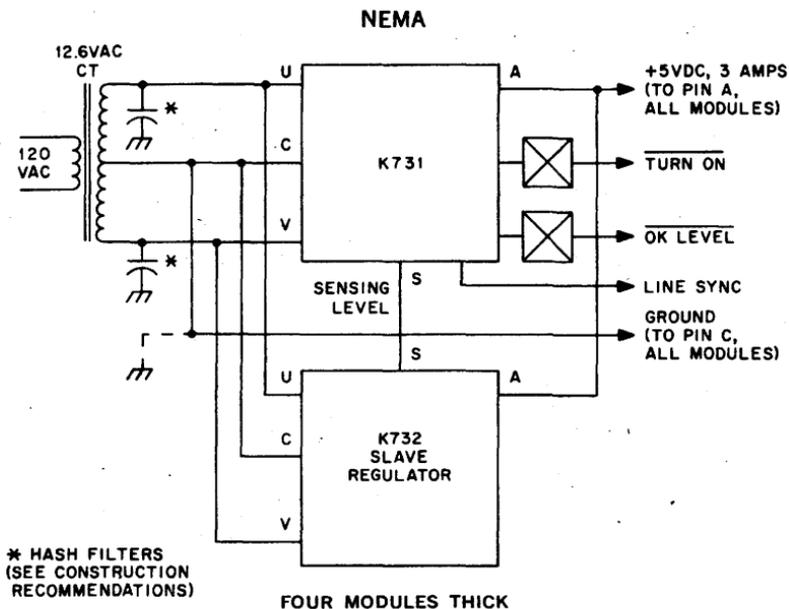
This module is normally tied to corresponding pins A,C,S,U, and V of a K731 Source. For each unit of current emitted by the K731, the K732 emits two. Up to three K732 slaves can be controlled by a single K731 for a total system current of 7 amperes.
