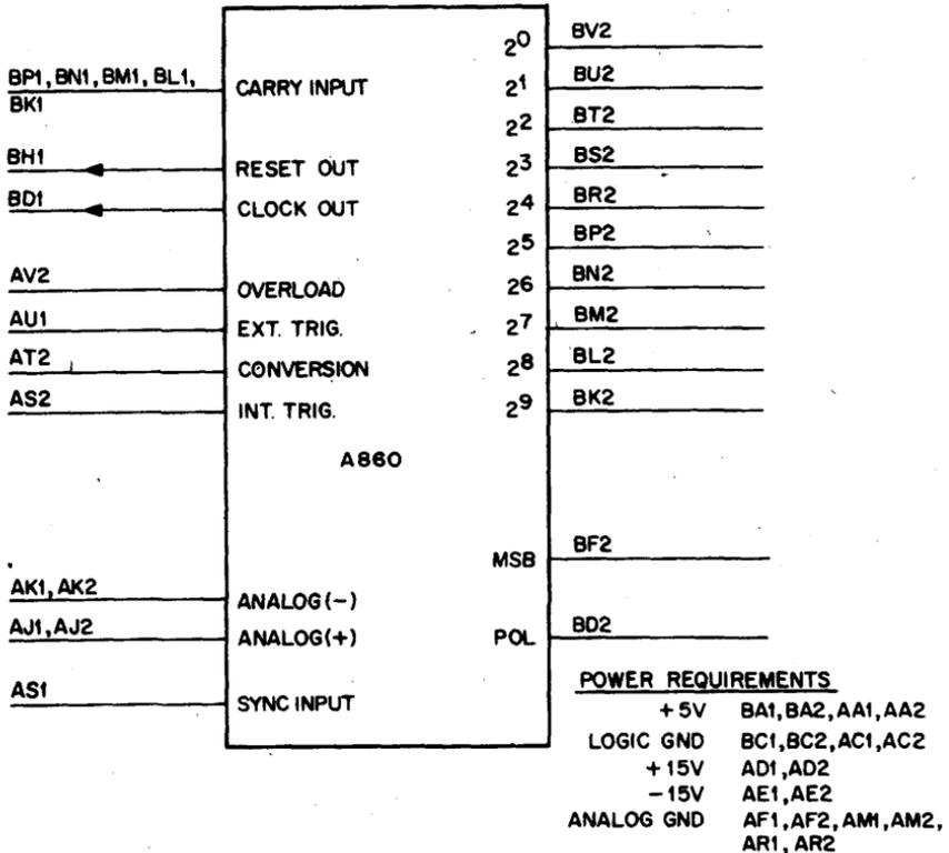
The A860 is a 12 bit industrial converter employing dual slope integrating techniques whereby an analog signal is converted into 12 bits (11 bits + sign) of digital information in 9 milliseconds.
