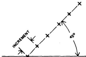
**BHC BOLT HOLE CIRCLE:** Allows for computation of bolt holes by specifying, in order, the radius of circle, angle from X axis of first hole, and number of holes.
