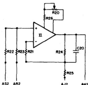
The A260 is a universal dual amplifier card which contains two independent operational amplifiers. Provisions have been made for mounting input and feedback components so that the A260 may be used in a variety of modes.
