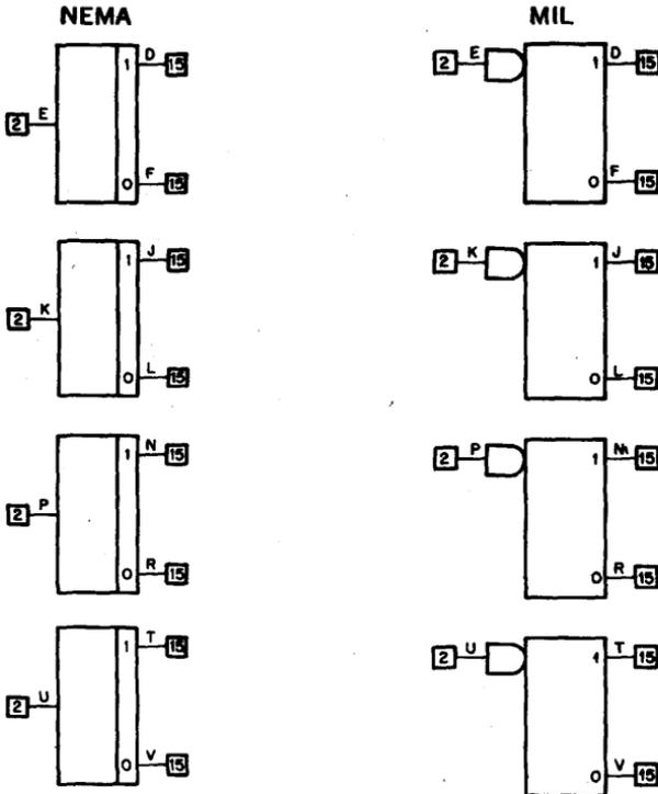
The K501 can be used with the K580, K581, or K578 to provide simultaneous true and complementary signals with full K series drive. Built in hysteresis and slowed outputs insure reliable operation in noisy signal environments.
