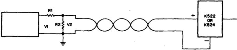
$R_2$  must be between 0 ohms and 20K for the K522, 0 and 100K for K524.  $R_1$  and  $R_2$  should be chosen so that  $\frac{V_1 \text{ (max)}}{R_1 + R_2}$  equal the maximum output
