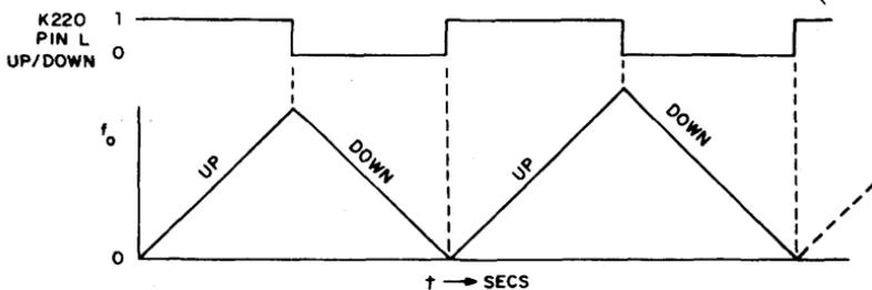
The response of  $f_o$  shown above is average and must be smoothed digitally to remove unacceptably large variations in pulse spacing; which would cause for example a Stepping Motor to change velocity instantaneously during the Acceleration period.
