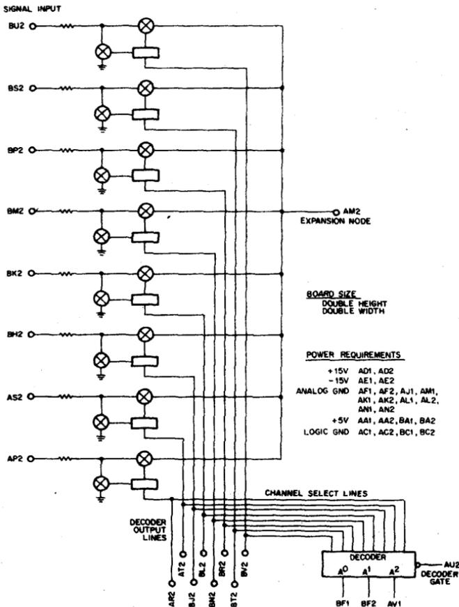
The A166 is a constant impedance eight channel multiplexer with decoder.
