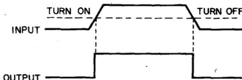
Some K Series modules, however, have a built-in feedback network which increases the voltage threshold necessary to switch from a low to a high output and decrease the voltage threshold needed to switch from a high to a low output. This results in a voltage gap between the turn on level and the turn off level, which is known as the hysteresis of the circuit.
