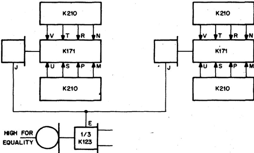
This module can be used in conjunction with the K174 to obtain the three independent outputs for greater-than, less-than, and equal-to.
