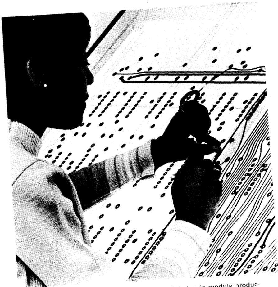
The printed circuit board layout is a crucial step in module production. Tolerances are checked to within  $1/5000$  of an inch.
