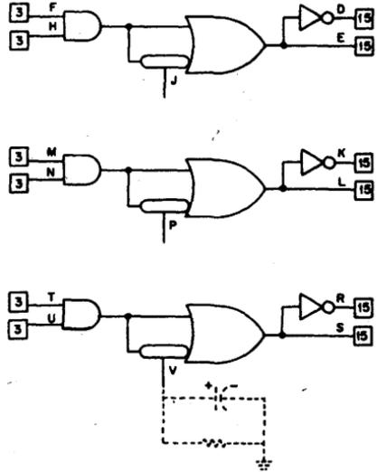
K303 timers provide time delays from 10 microseconds to 30 seconds and can be interconnected to form clocks with periods covering the same intervals. Fixed or adjustable delays and frequencies are obtainable. Calibrated controls are available (K371 through K378) for mounting directly on the K303. Remote controls can be added, if desired. A simplified schematic of the K303 is shown below. Note that the comparator has hysteresis, increasing the rejection of false "1" noise peaks at the input.
