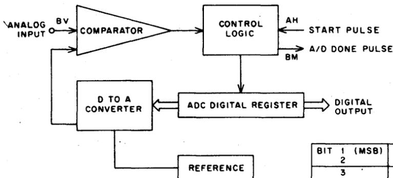
A801 10-BIT ANALOG-TO-DIGITAL CONVERTER
