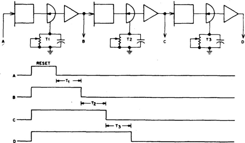
A pushbutton, clock, or another sequencer can provide signal A that resets all timers and begins the sequence. Any number of timers may be cascaded, but if many steps are needed one of the less flexible sequencers should be considered as a means of reducing the number of adjustments and the cost.
