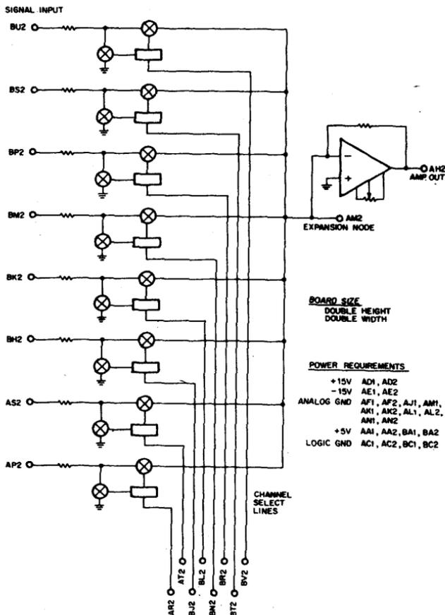
The A165 is a constant impedance multiplexer consisting of eight independent channels which utilize FETS to switch the input signal through precision resistors into either a ground (OFF) or a virtual ground of an operational amplifier (on).
