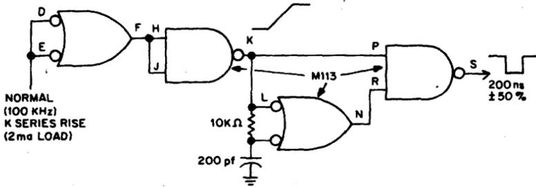
Note: Same input restrictions as K to M Series level converter. M113 may be replaced by M602 circuit if desired.
