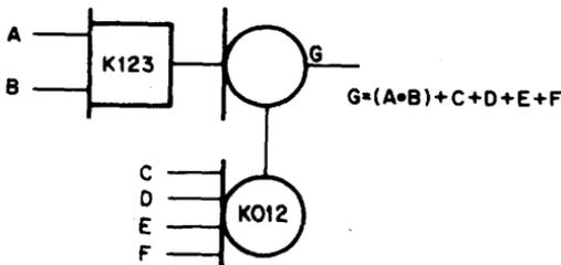
The K003 can be connected to the OR expansion input as follows:
