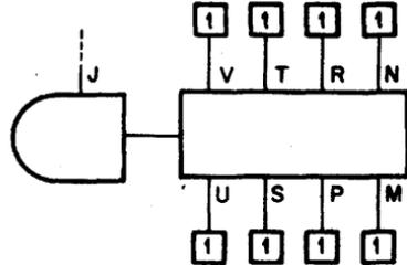
The K171 is a four bit equality comparator whose output at pin J is high if the two numbers being compared are equal. Pins N, R, T, and V are compared with pins M, P, S, and U. The output, Pin J, has no drive capability and must be connected to the AND expansion node of either a K113 or K123 logic gate.
