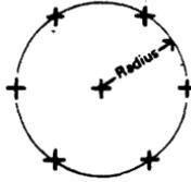
**ARC ARC:** Allows for computation of holes along an arc by specifying, in order, the radius of arc, angle from X axis of first hole, incremental angle between holes, number of holes.
