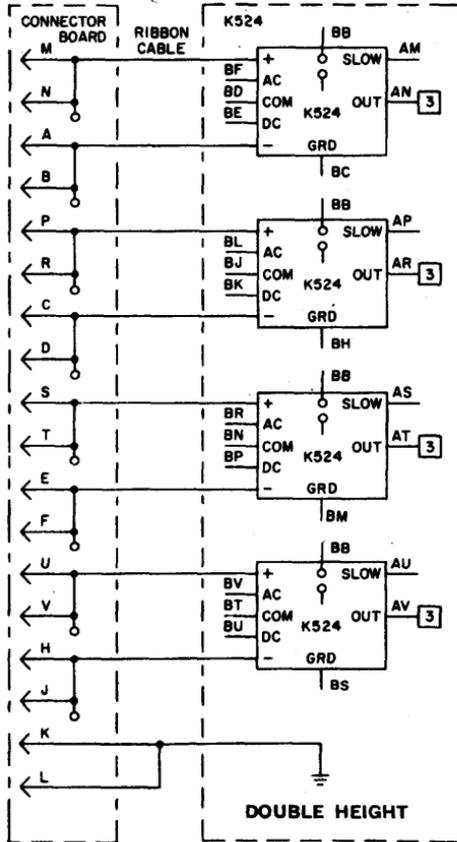
Basically a noise-rejecting, threshold sensing differential voltage amplifier, the K524 is readily adapted to sensing threshold points in DC analog signals, AC signals, and pulses. It can also be biased to sense resistance thresholds. The differential amplifying technique permits flexible grounding and shielding methods to accommodate floating signal generators and minimize noise.
