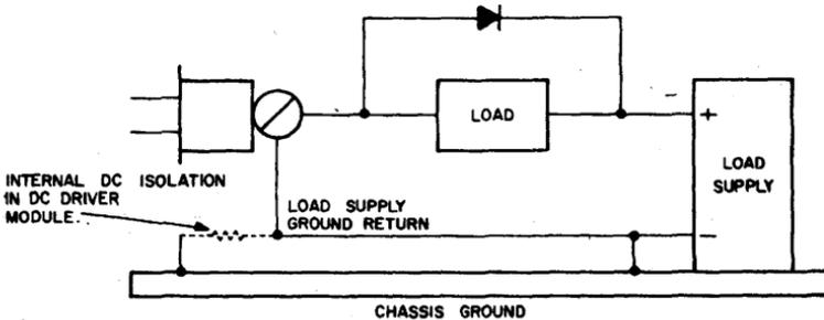
**NOTE:** If the ground return wire is not provided, current will have to flow through the chassis ground.
