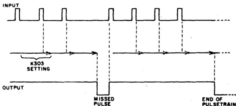
Input signal can be a square wave or pulses of any width down to 0.3% of the maximum delay available with the timing capacitor used. (Pulsewidths down to 0.1% or less may be used if timing consistency can be sacrificed). Timer delay would normally be set 30% to 50% longer than the nominal pulse repetition rate to detect missed pulses in a train, or at the geometric mean between two pulse periods which are to be distinguished.
