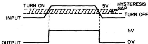
Those K Series modules which contain hysteresis have voltage gaps from .5 to 1 volt in width, resulting in a higher voltage threshold necessary to turn the circuit on. As an example: suppose a circuit turns on at 2.4 volts and turns off at 1.4 volts, then it would require a noise spike 2.4 volts high and 1.5 microseconds wide to trigger a false high level. To be falsely interpreted as a low level, a high level (+5) would now have to drop 3.6 volts for 1.5 microseconds.
