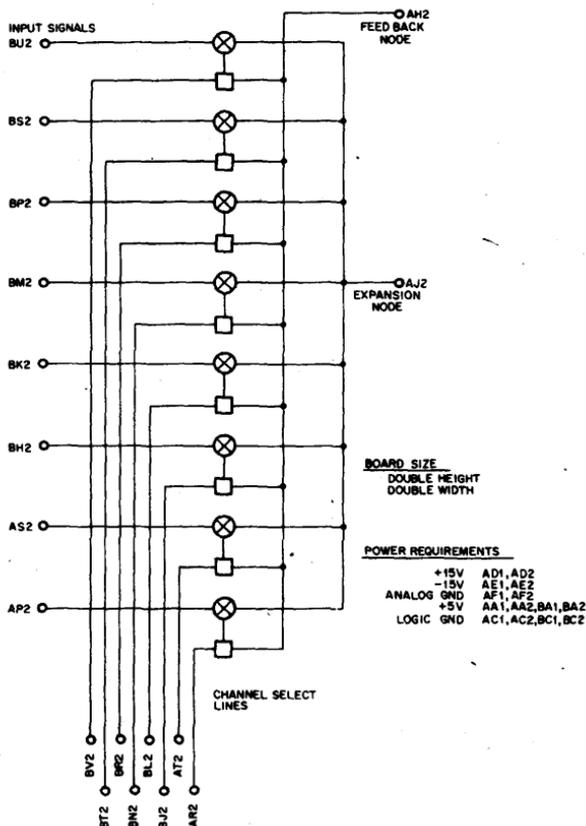
The A160 is a high impedance multiplexer expander consisting of 8 independent FET channels.
