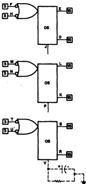
K323 one shots provide output pulse widths from 10 microseconds to 30 seconds with either fixed or adjustable delays. Calibrated controls are available (K374, K376 and K378) for mounting directly on the K323. Remote controls can be added, if desired.
