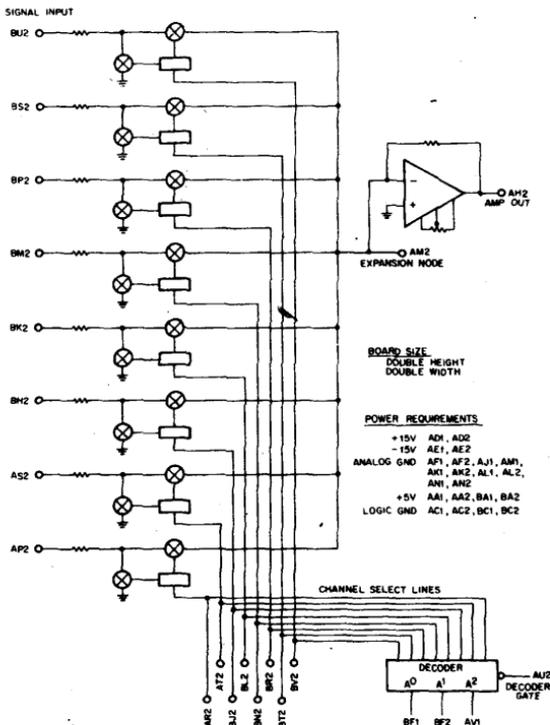
The A167 is an eight channel constant impedance multiplexer with output amplifier and decoder. The operation of the A167 is performed in the same manner as any of the other DEC constant impedance multiplexers, where the input signal is switched via FETs to either ground (OFF) or into a virtual ground null point (ON) of the operational amplifier.
