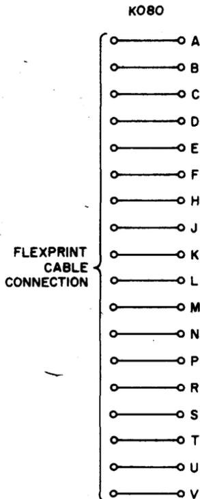
The K080 cable connector consists of a single height, single thickness board on which can be mounted a 19 conductor flexprint cable. Each module comes with a cable clamp for customer convenience.
