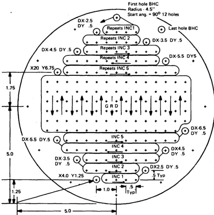
192-Hole Drilling Application for Quickpoint
