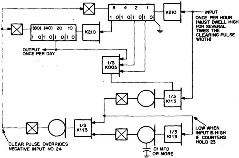
The basic principle involved is to detect the largest number to be permitted, and to generate a clear pulse when it disappears due to the reception of one more count. The same method may be extended to counters of any length, provided the clear pulsewidth is wide enough to override any possible carry propagation.
