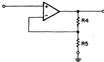
$$\frac{E_O}{E_{IN}} = \frac{R_4 + R_5}{R_5}$$
