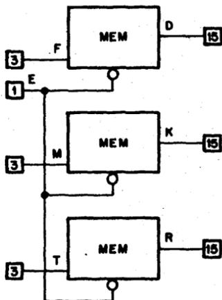
Three magnetically latched mercury wetted contact relays in the K273 follow logic-level input information at rates up to 100 Hz, when pin E is grounded.
