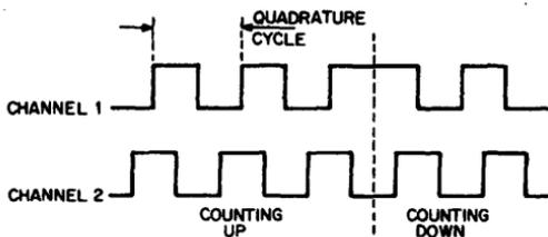
For counting up channel 2 leads channel 1 by 1/4 cycle and for counting down channel 1 lead channel 2 by 1/4 cycle. The channel which leads for UP and DOWN counting is determined by the type of quadrature encoder used and how it is wired to the K531. If the unit does not count properly, the quadrature inputs to the K531 may need to be switched.
