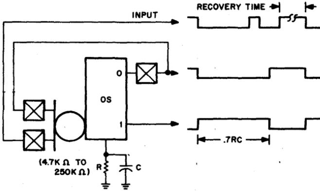
A positive pulse at the input will not terminate the timeout if one input is connected to the oneshot inverted output (either pin D,K, or R).
