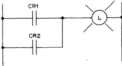
In this circuit, the light is on when either or both contacts CR1, CR2 are closed. This is the OR function  $L = CR1 + CR2$ .
