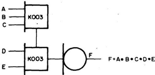
Up to 100 inputs may be connected to the AND Expansion input.
