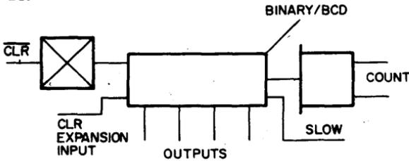
The K220 is a binary or BCD up/down counter which can be parallel loaded. With these two counters, virtually any counting function can be easily implemented.
