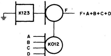
Up to 9 "OR" inputs can be connected to the OR expansion input.
