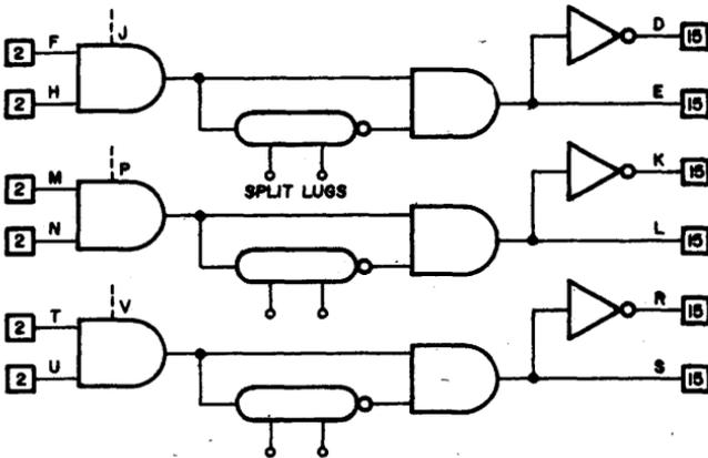
The K333 Pulsers circuits are designed to produce pulses from low to high level transitions. The length of a pulse is determined by the capacitance connected to split lugs conveniently mounted on the module.
