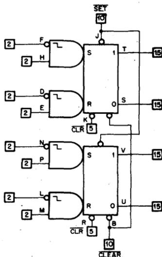
This superslow memory simplifies sequencing of machine motions, and finds other applications where the ultimate in noise isolation is needed and speed is no problem. Its 1 KHz maximum repetition rate makes this flip-flop noticeably more resistant to extremely noisy surroundings than faster types like K202, K210, etc. So noise immune, in fact, that several yards of wire may be connected to K201 outputs even in severely noisy areas without errors.
