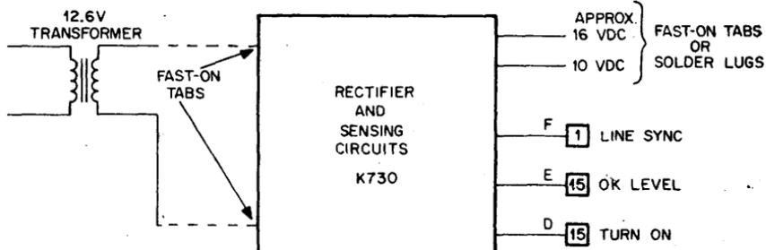
The K730 is a general purpose module that can be used with any +5 volt power supply to generate the turn on and power OK signals that are normally provided by the K731.
