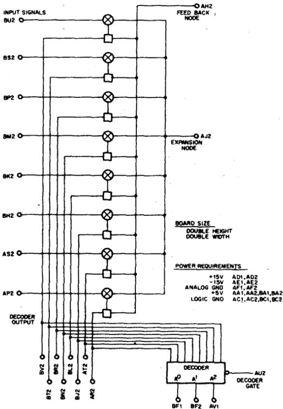
The A162 is a high impedance multiplexer with decoder consisting of 8 independent FET switched channels. Included on this module is a gated binary to octal decoder for selecting any of the eight high speed channels.
