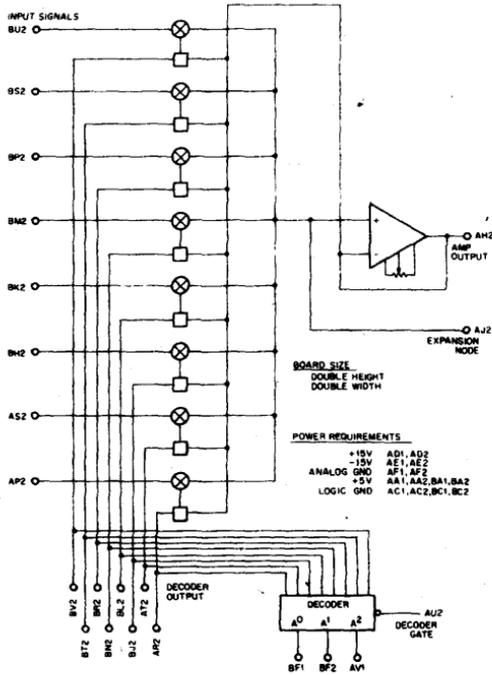
The A163 is a high impedance multiplexer consisting of 8 FET switched channels, a noninverting unity gain follower amplifier, and an 8 bit binary to octal decoder for channel selecting.
