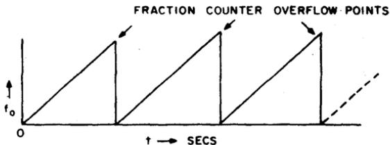
Resolution can be increased by module cascading. If the Fraction Counter is a K220 UP/DOWN Counter connected for Binary operation,\* then the slope of  $f_0$  can be reversed and controlled symmetrically.
