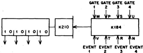
**USING K184 TO GENERATE EVENT COMPLETION PULSES**
