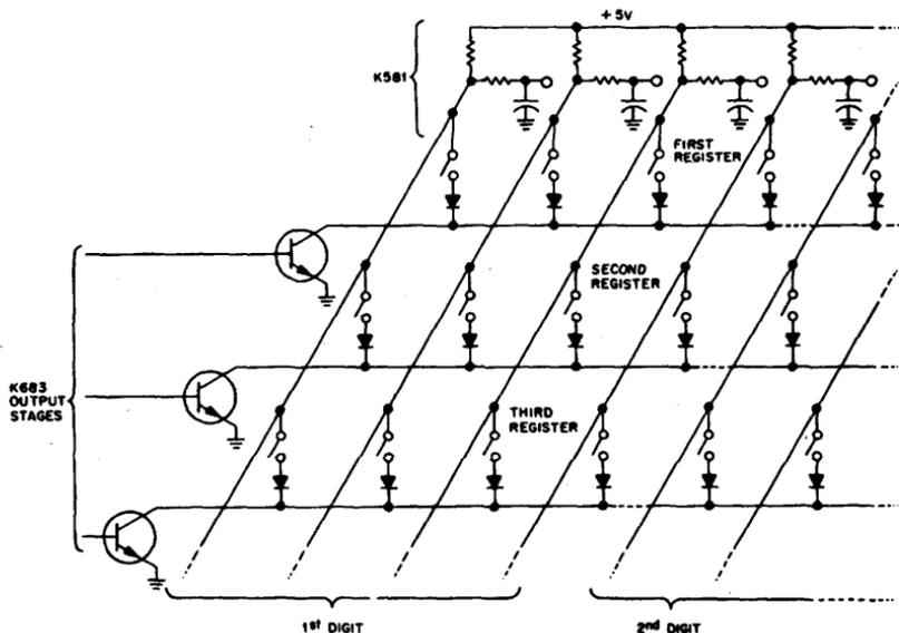
To sequence through the registers, it is necessary to turn on one K683 circuit at a time; this can be done by a K161 binary to octal decoder. Since no BCD decade can draw more than 60 milliamperes, as many as four decades can be handled on any one K683 switch. Circuits may be paralleled for larger registers.
