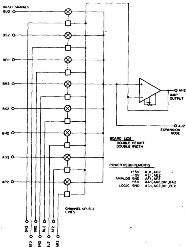
The A161 is a high impedance multiplexer consisting of 8 independent FET switched channels and a noninverting unity gain follower amplifier, designed for application where accuracy, high speed, and high input impedance are prime requirements.
