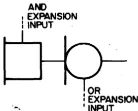
The "AND" expansion input is used with the K003 AND Expander, to provide the AND or NAND function for more than 2 inputs. For example, with one K003 AND Expander connected to a K123 Non-inverting gate we create a five input AND gate.
