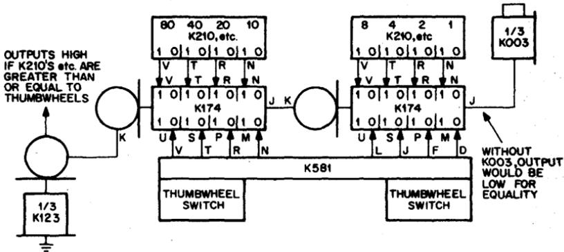
If the numbers being compared are not multiples of 4 bits then one of the inputs on each unused comparator position must be connected to +5 and the other one to the ground.
