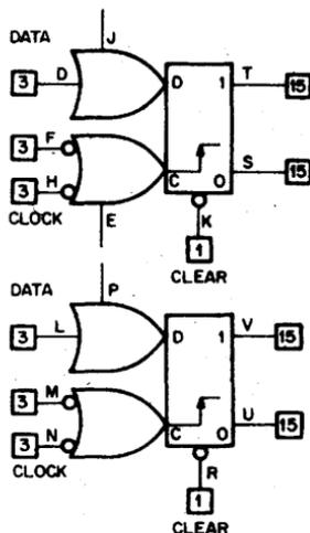
K202 flip-flops do shifting, complementing, counting, and other functions beyond the capabilities of simple set-reset flip-flops built up from logic gates. They also may be used to extend K210 counters or K230 shift registers.
