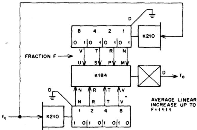
As shown below, if the FRACTION K210 overflows from 1111 to 0000,  $f_0$  will fall to zero and begin again to increment as before. The result is a Digital Sawtooth generator.  $f_0$  against time  $t$  is shown here.
