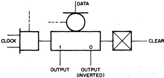
The D type flip-flop output goes to the state of the D input when the clock input falls from high to low. Notice the built in gates with expansion inputs on the clock and Data inputs. These allow simple input conditioning.
