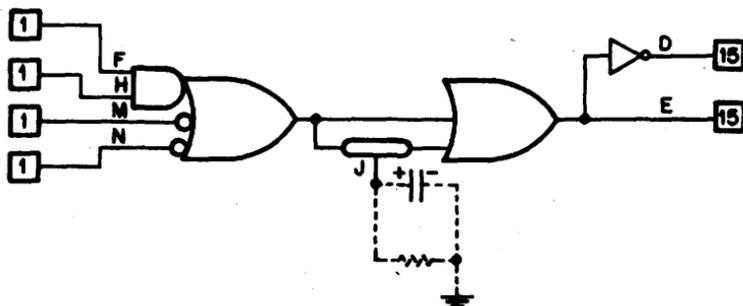
The K301 Basic Timer can be used as an OFF DELAY (like the K303), ON DELAY or ONE SHOT (like the K323). Time delays from ten microseconds to 30 seconds can be obtained with either fixed or adjustable delays. Calibrated controls are available (K374, K376 and K378) for mounting directly on the K301. Remote controls can be added if desired. Mounting holes are provided on the module for different size timing capacitors and a trimpot or fixed resistor.
