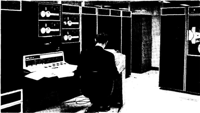
DEC's large PDP-10 computer, a portion of which is shown here, is used in application ranging from financial management to commercial time-sharing to plant monitoring.
