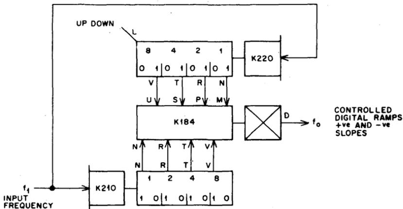
The output of the K184 shown above, is on the average, a linearly increasing frequency when the K220 counts UP, and a linearly decreasing frequency on K220 count DOWN. This facility is of use in controlling Stepping Motor Acceleration on K220 UP counts, and Deceleration on DOWN counts. The Fraction Counter must not be allowed to overflow.
