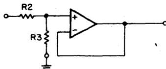
$$\frac{E_O}{E_{IN}} = \frac{R_3}{R_3 + R_2}$$
