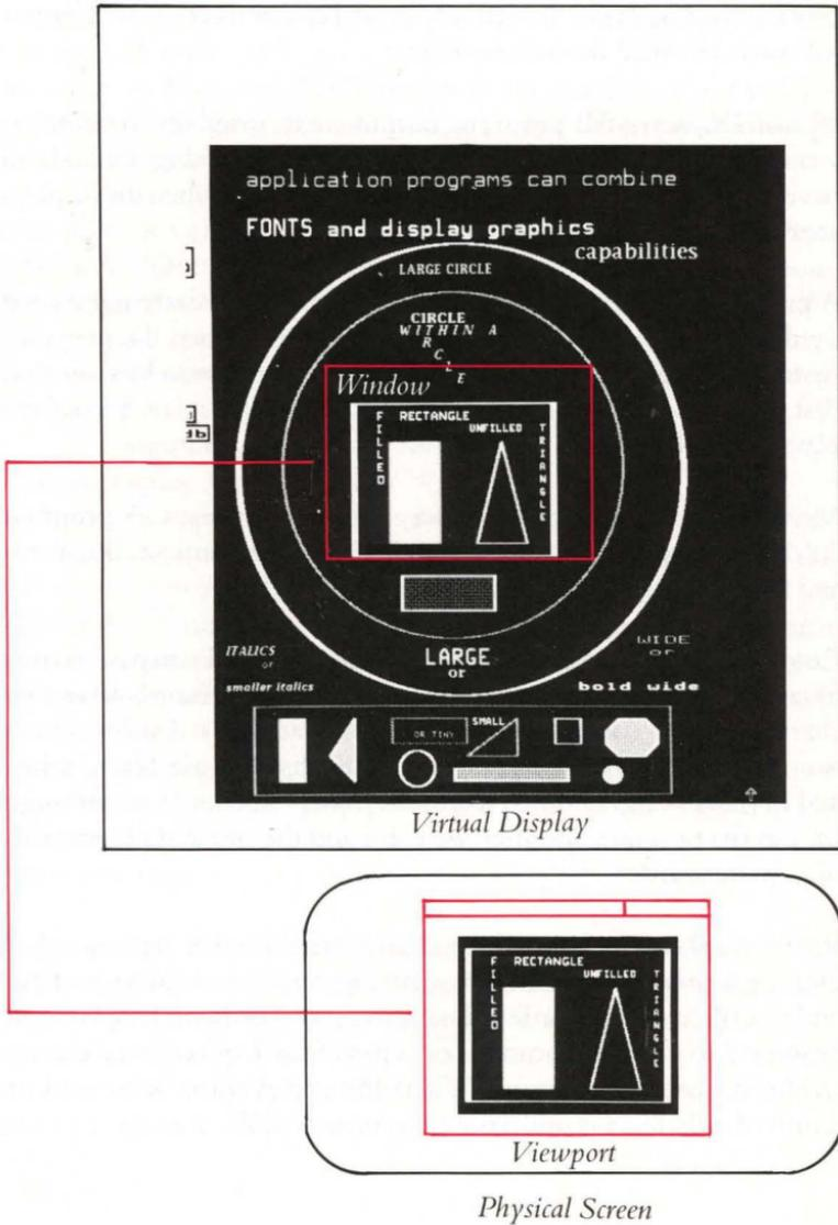
Pasteboards are both output devices and input devices. As output devices, they define the spatial relations of virtual displays and windows. As input devices, they define the location of the pointer on the screen that is meaningful to a program, and determine which process can read user input from the mouse, keyboard, and optional graphics data pad.
