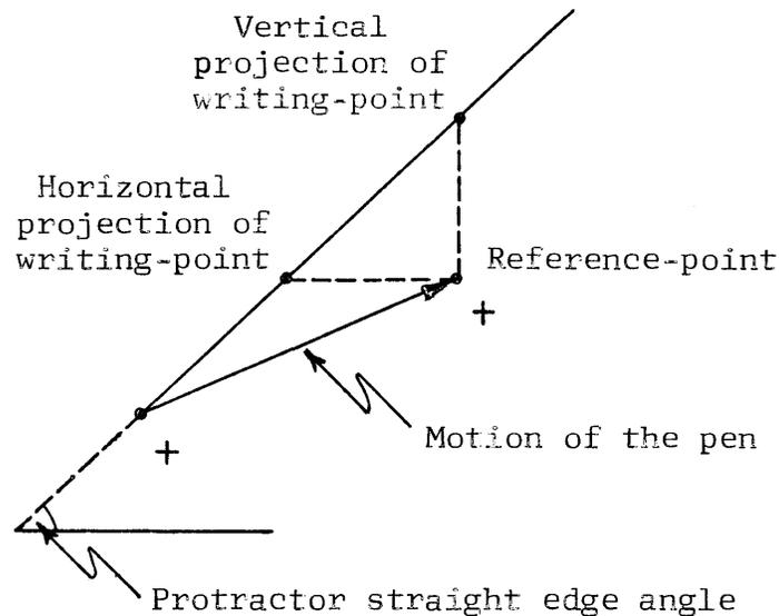
The reference-point in the two illustrations above greatly reduces the need for guide lines. Furthermore, the ability to interrupt tracking long enough to use the pen as a pointer for the reference-point provides an effective drawing ability. This is done by depressing the LOCK-ON push button, which causes the Pick routine to be activated in choosing an existing point on the drawing.
