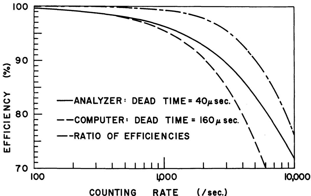
Figure 8 Efficiency curve for multichannel pulse-height analyzer as a function of stored counting rate for:
