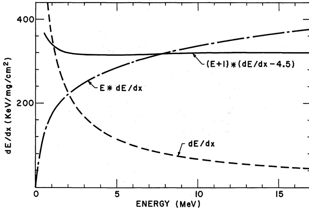
Figure 5 Variation with energy  $E$  of incoming particle of
