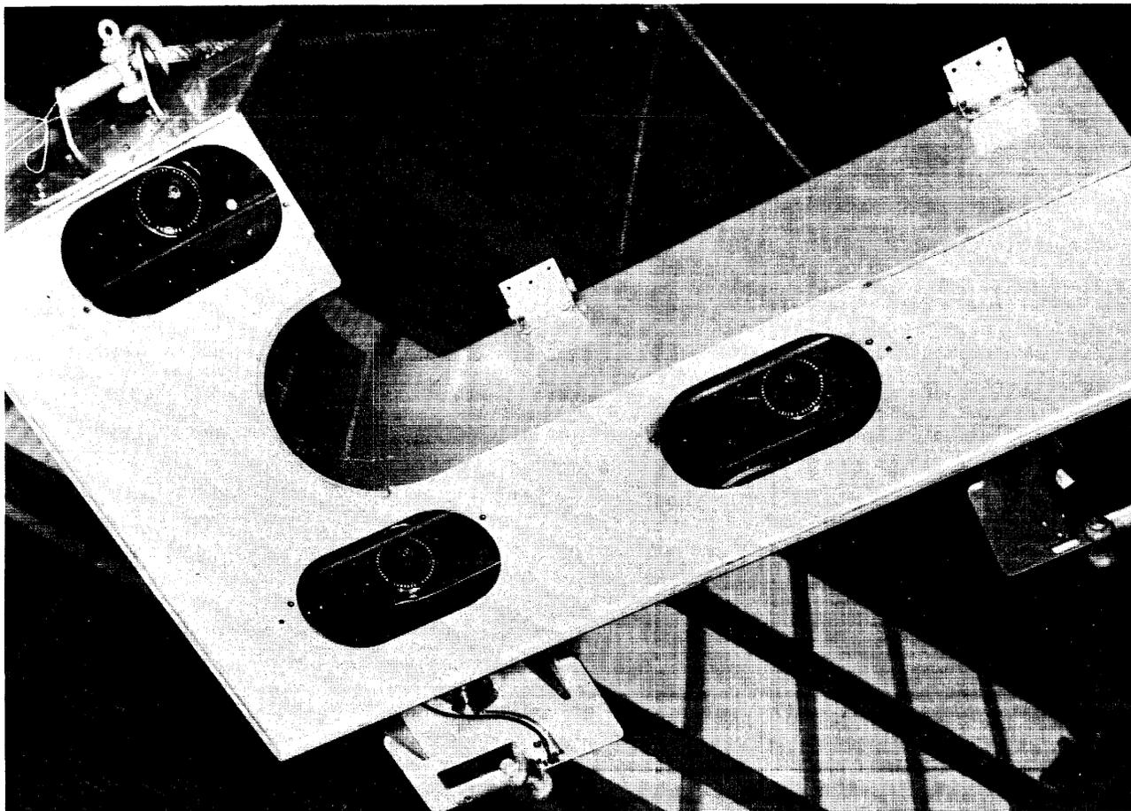
Figure 2 Three Bubble Chamber Cameras
