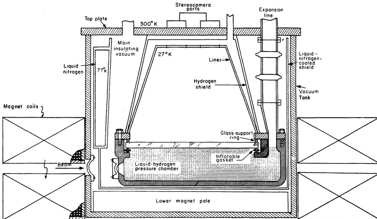
Figure 1 72-Inch Bubble Chamber
