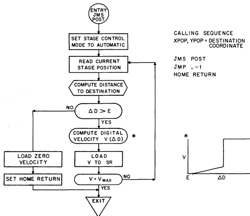
Figure 13 Stage Position Subroutine Flow Chart
