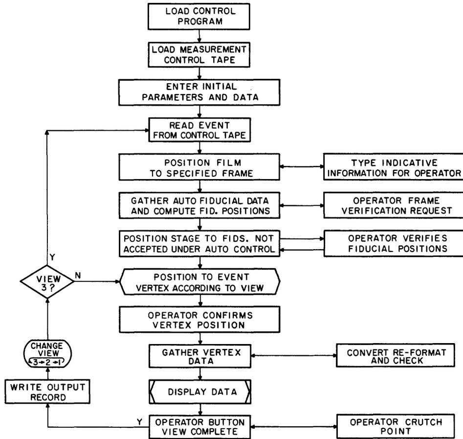
Figure 14 Normal Program Sequence for Single Vertex Events
