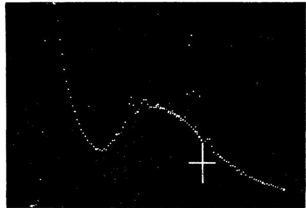
Figure 11 Pulse-height spectrum of gamma rays incident on a Li-drifted Ge solid state detector illustrating real-time determination of background (smooth curve under prominent peak)
