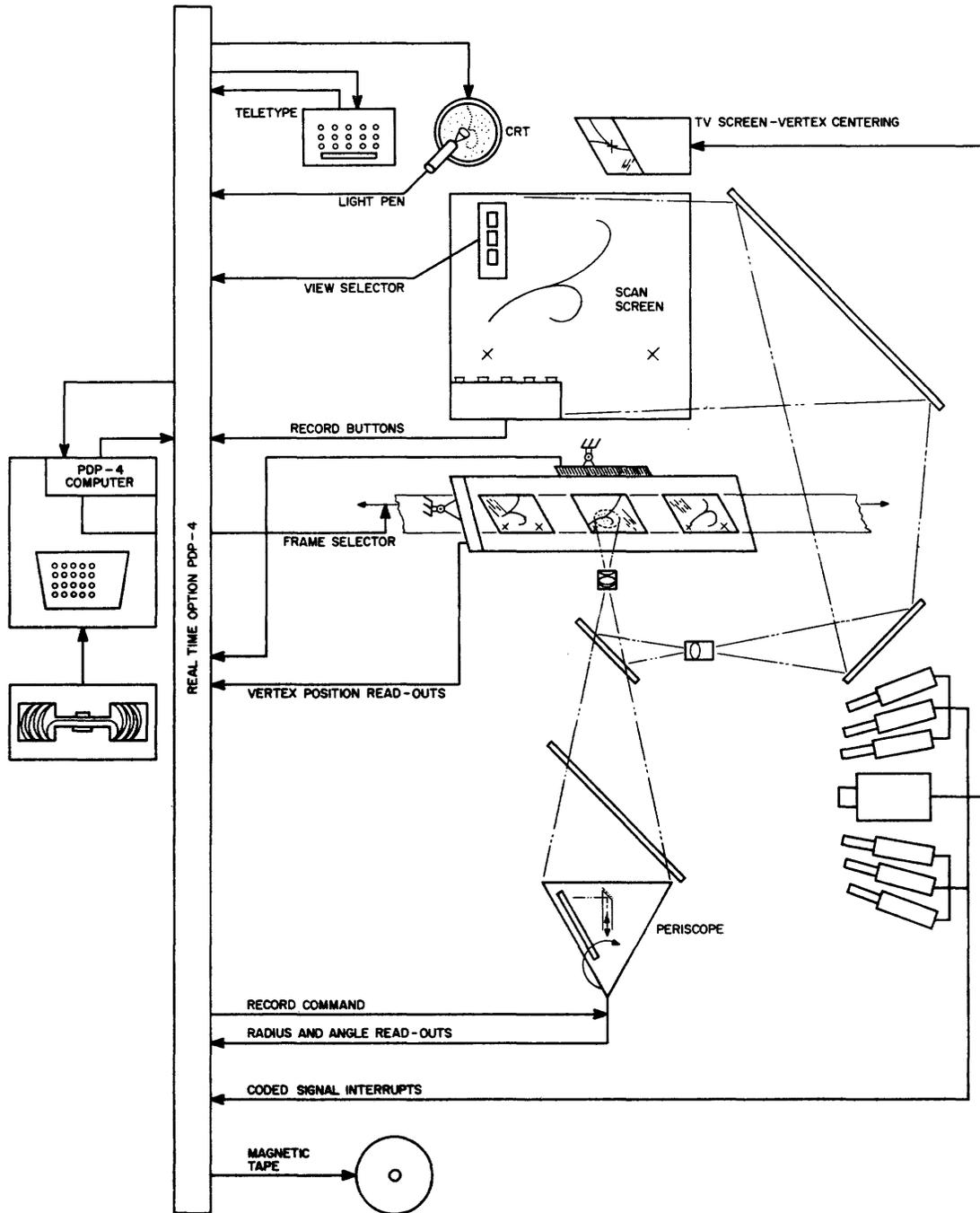
Figure 10 Information and Control Sequence Measuring Projector
