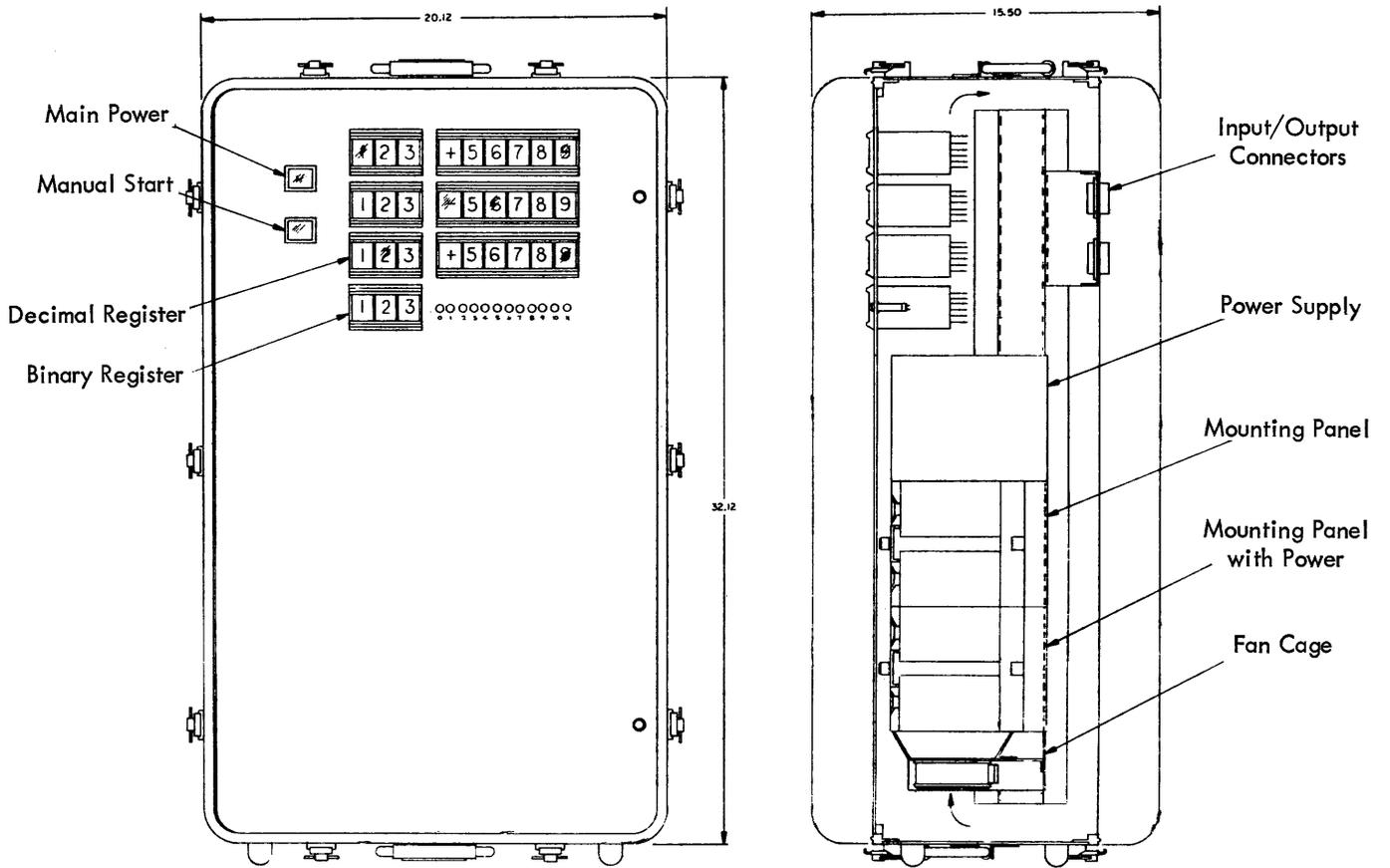
Figure 4 14 Containers of the Overall System
