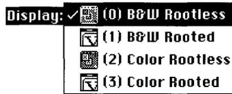
The screen number (0 through 3) preceding each screen type represents a style (rooted or rootless) and a type of screen (color or black and white). In the previous illustration, the display chosen is number zero (0), which specifies a black-and-white screen in which the root window does not appear (rootless). MacX will display the client window on the largest video monitor that fits the screen type selected.
