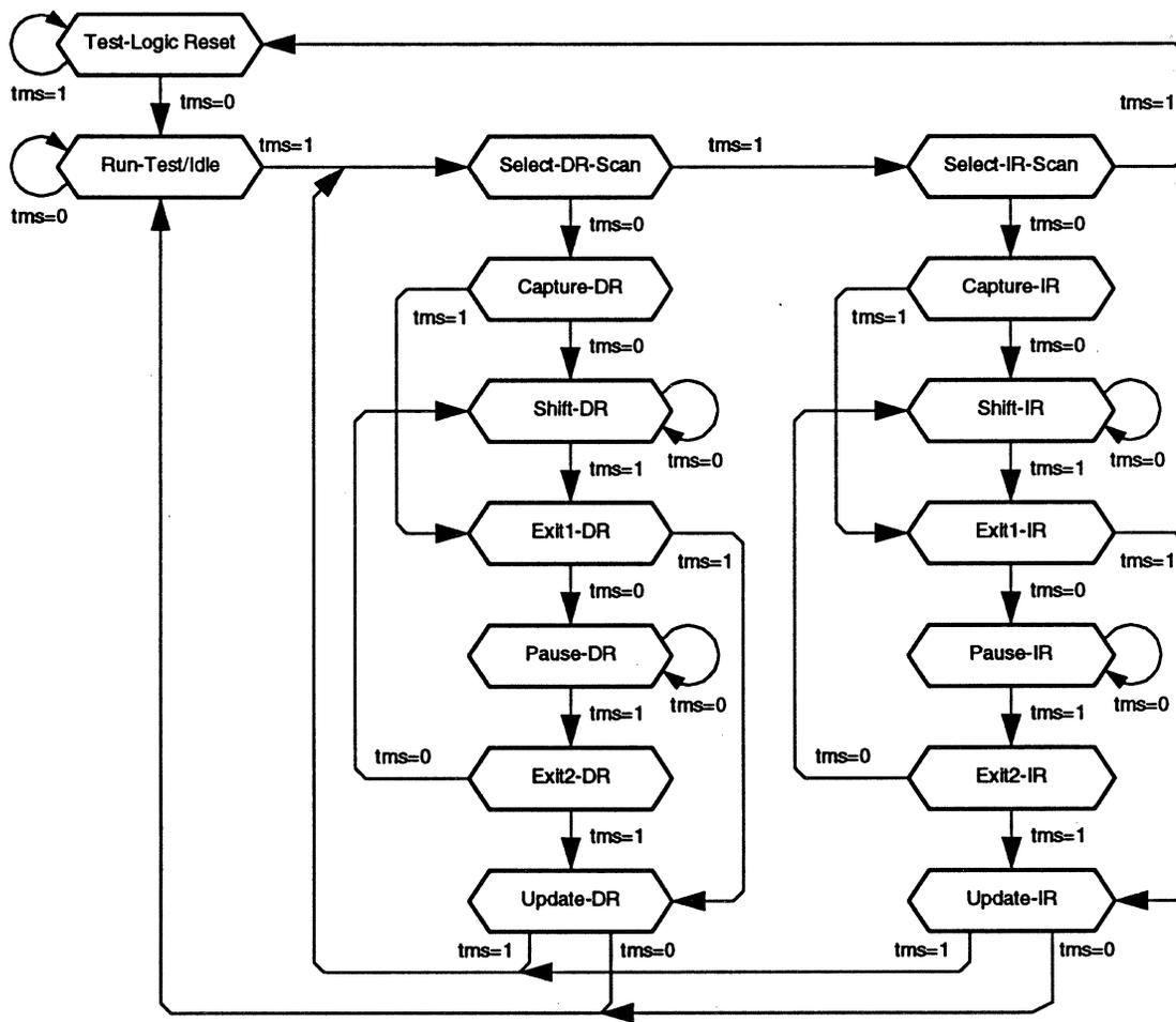
Figure 49: Test Access Port (TAP) Controller State Transitions
